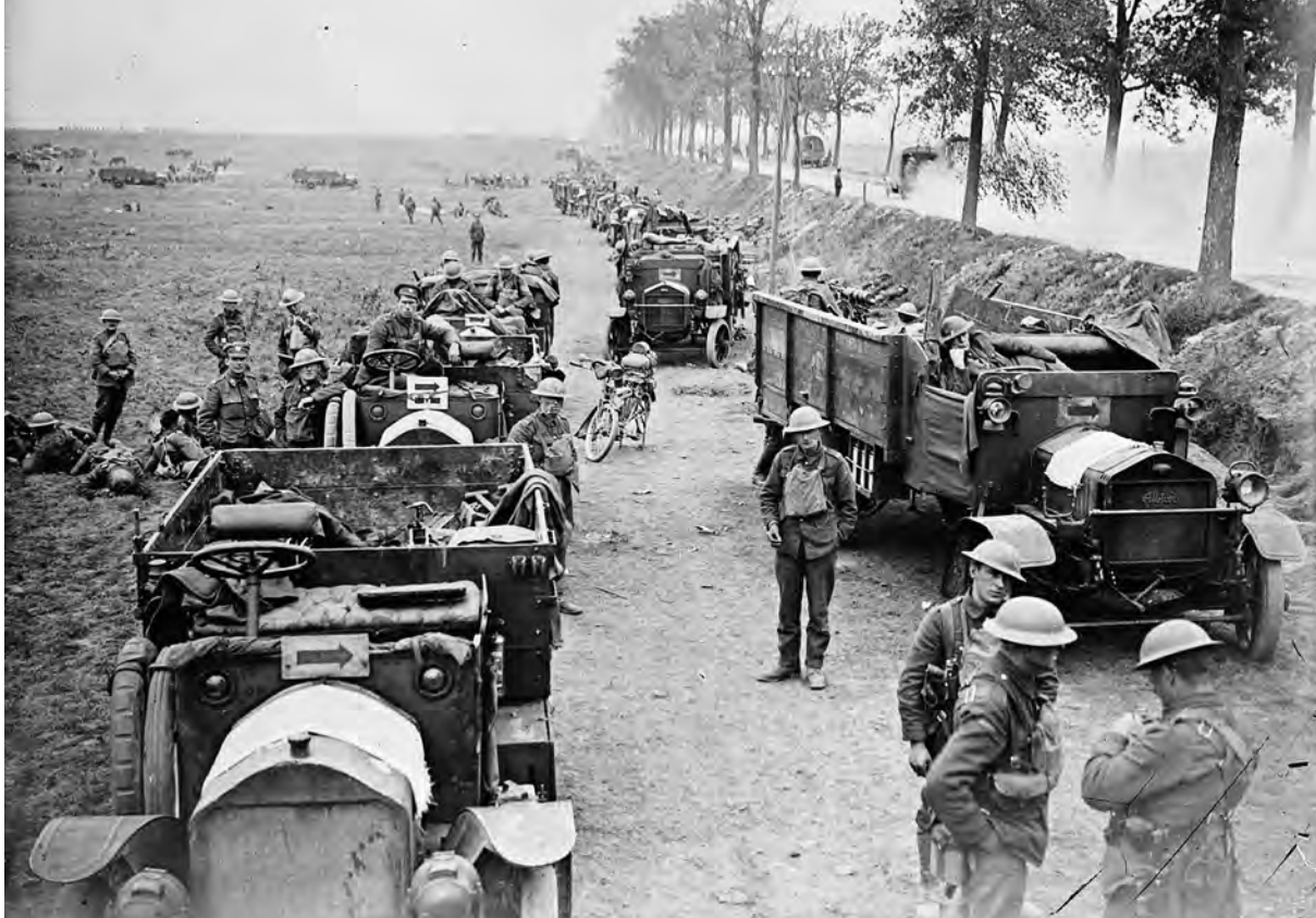
A Canadian Motor Machine Gun Brigade waiting alongside Arras–Cambrai Road. Advance east of Arras, September 1918. By June 1918 onwards, 6 of the 8 original “Auto Car” armoured cars remained. Each of the CMMGB was equipped with 20 of these “Auto Car Lorries.” Clearly visible on the back of the right-hand vehicle is the Vickers HMG on the pedestal mount manufactured by the Canadian Motor Machine Gun Mechanical Transport Company. Library and Archives Canada, PA-003399.
