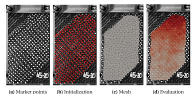
Figure 7.16: Steps for DIC analysis. (a) The specimen is prepared with white marker points. (b) The tracking points are identified in the initial frame. (c) The resulting deformed points are interpolated by Delaunay triangulation (d) The displacement field is interpolated with shape functions and deformation measures are evaluated on the evaluation mesh.
