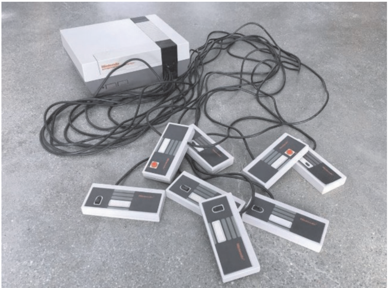
Figure 5: The Octopad by Patrick LeMieux. This modified NES has eight controllers that function as one, as each has only one of the standard eight NES buttons: A, B, Up, Down, Left, Right, Select, and Start. Photo credit: Patrick LeMieux.
