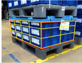
Figure 1.1: Illustration of Packaging Structure Recognition. Transport unit side faces are illustrated in red, yellow lines indicate packaging unit rows and columns.
