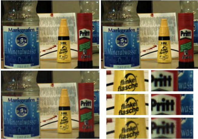
Figure 4.1: Center views of the light field. Dansereau et al. (top left), Bok et al. (top right), proposed method (bottom left). Detailed views: Dansereau et al. (top), Bok et al. (middle), proposed method (bottom).
