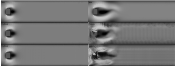
Figure 4.1: 1. Line: Step 1 and step 20 of a finite element simulation, 2. Line: Predicted step 1 and step 20 without the usage of the pressure field, 3. Line: Predicted step 1 and step 20 with usage of the pressure field; No binary mask used, x-velocity shown
