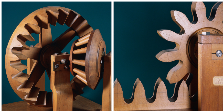
Fig. 16 Wooden models of gearings designed by Théodore Olivier for his teaching at the Conservatoire. © Musée des arts et métiers-Cnam, Paris/photos P. Faligot, all rights reserved
