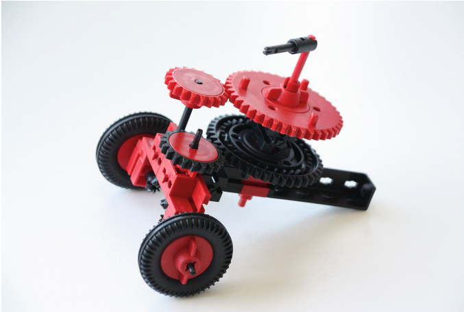
Fig. 7 Model of a south-pointing chariot realized with Fischer-Technik according to a design by Thomas Püttmann. © Photo: Tilman Sauer, all rights reserved
