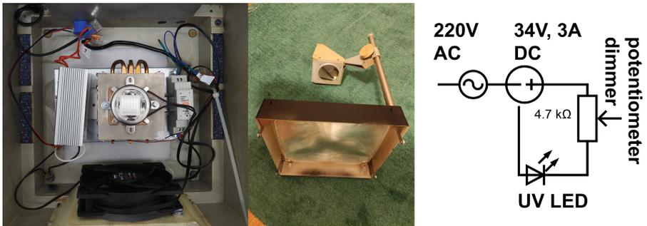
**Fig. 3.** Left: modified overhead projector with UV LED, Middle: overhead projector optics (Fresnel lens and adjustable mirror), Right: electrical schema.
