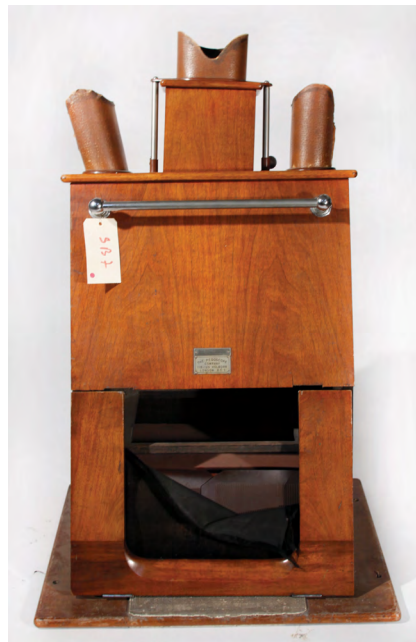
Figure 2.2: X-ray shoe-fitting device. The customer stood holding the bar while placing their feet in the dark opening. An X-ray source below the feet enabled the customer, salesperson, and a third person to view the foot bones from above. This particular machine was manufactured by the Pedoscope Company of London and is housed at the museum of the University Hospital of Lyon, France. Photographers: Roxanne Poudenas and Léo Lespets. https://commons.wikimedia.org/wiki/File:Podoscope_par_The_Pedoscope_Compagny_01.jpg . CC BY-SA 4.0.
