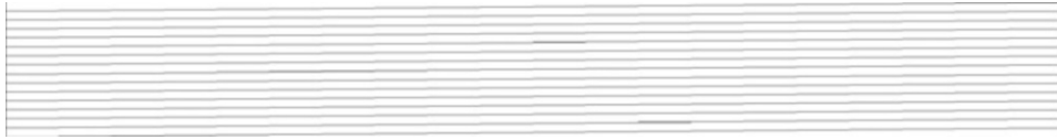
Fig. 3 Pattern to identify 300 nozzles of a thermal inkjet print head. Every twentieth nozzle is firing in vertical direction. In horizontal direction for the next partial pattern the number is increased by one. A vertical line is positioned in the leading and trailing column
