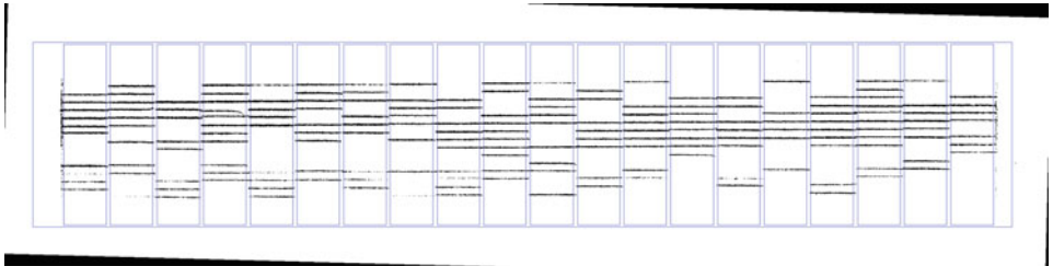
Fig. 7 The rotated pattern image including the outer frame used to optimize the rotation and 20 frames to identify groups of nozzles
