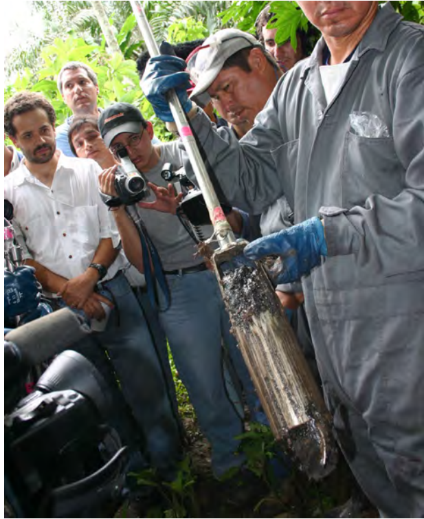
FIGURE 11 An auger soil core from the judicial inspections at Sacha Sur. Photo © Amazon Watch. Used with kind permission.
