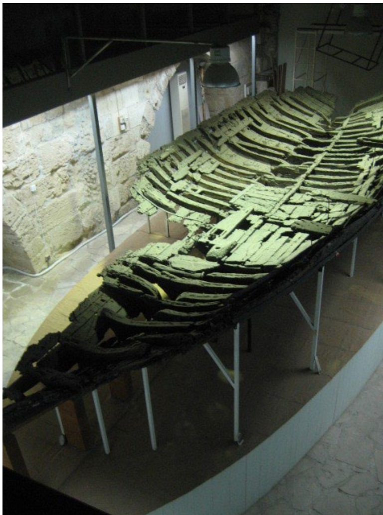
Figure 41: The original wreck at Kyrenia castle. It was built in the shell-first method and for its construction some 8,000 mortises have been cut to receive 4,000 tenons, providing a very rigid construction before any internal framing (courtesy Department of Antiquities, Cyprus).
