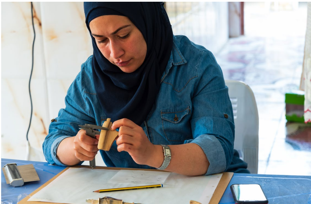
Figure 22.14 Measuring sherd thickness with callipers
