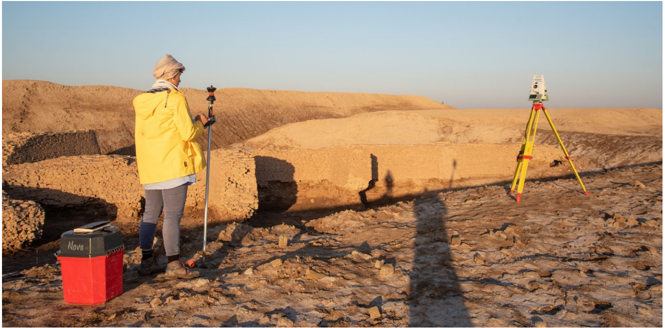
▲ Figure 7.4 Survey using a multi station by one person using the remote function
