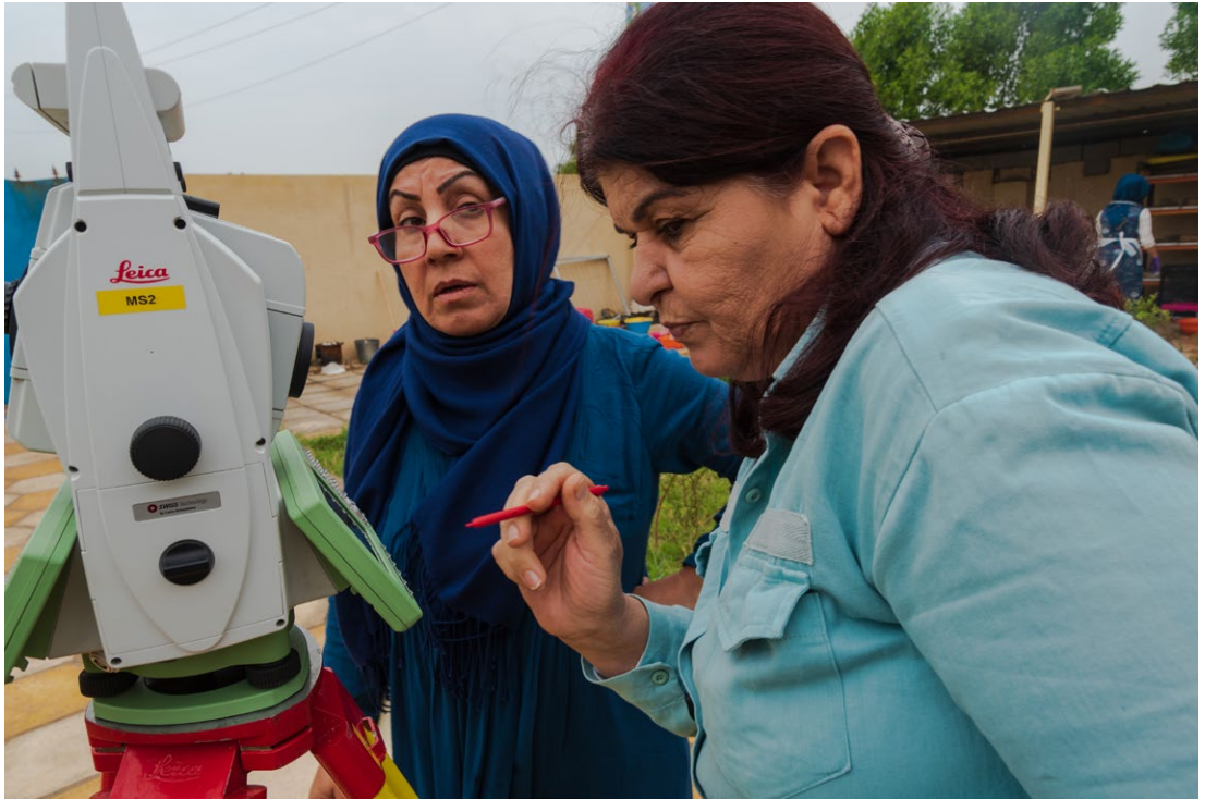
Figure 7.7 Using the control screen on a multi station
