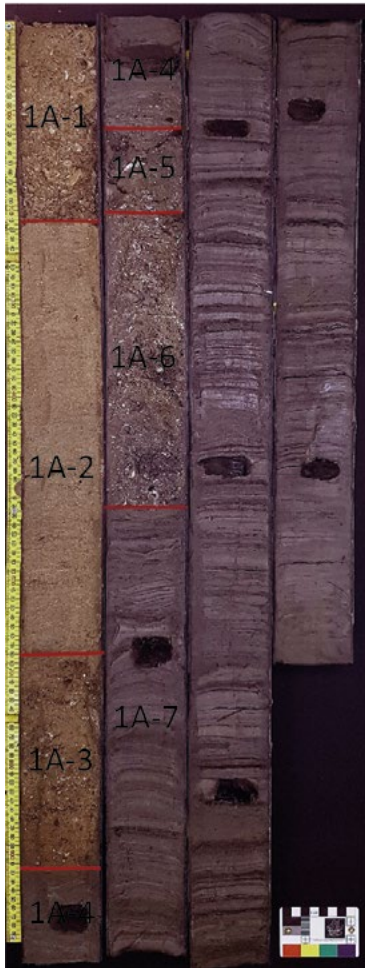
Figure 12.4 Sampling strategy for ELF cores – illustrated with core ELF001A: (a) core, with sub-units identified; (b) core, with sampling positions indicated; (c) removal of sediment for OSL profiling, OSL dating and dosimetry.
