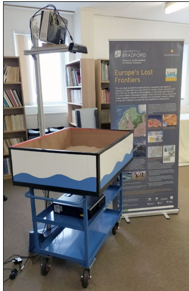
Figure 14.6 The ELF Augmented Reality sandbox.
