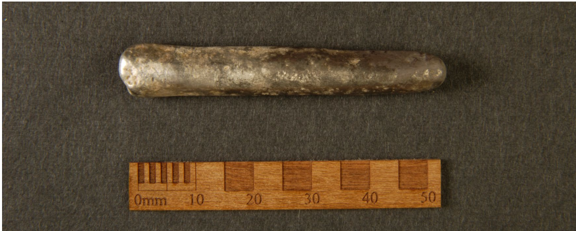
Figure 2.26. Ingot with both silver chloride and silver sulphide corrosion (AN2017.12; cat 1.5).
