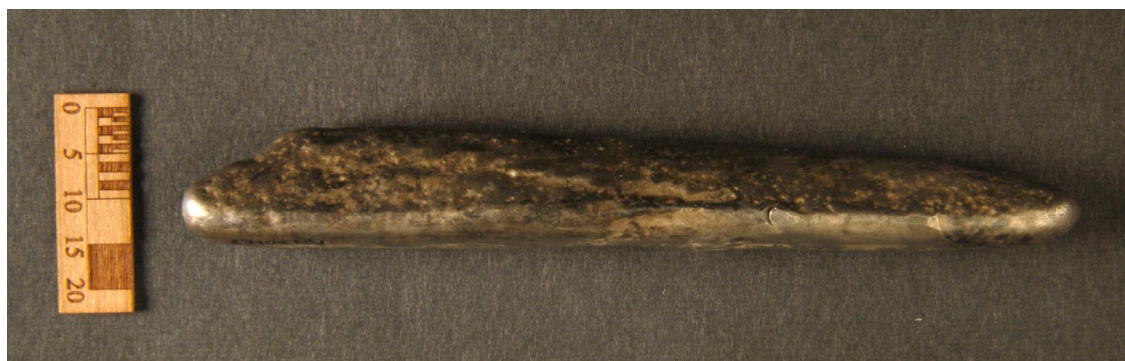
Figure 2.29. Ingot (AN2017.8; cat. 1.1) after cleaning. Note the nicks along the edge of the ingot.
