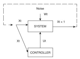
Figure 10.3 Standard schematic for an inherently unstable control system. The system output at time t + 1,  $X_{t+1}$  is a function of output at the previous time t, added noise,  $W_t$ , and the control signal at time  $t U_t$ . The controller samples the output at time t, compares it with an internal picture of the world, and then makes corrections as needed.
