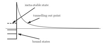
Figure 6.5. A nuclear tunnelling potential
