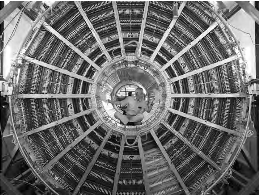
Figure 10.18 Front view of the ALICE TPC end-plate, with the technical coordinator, Peter Glassel. Picture CERN (2006).
