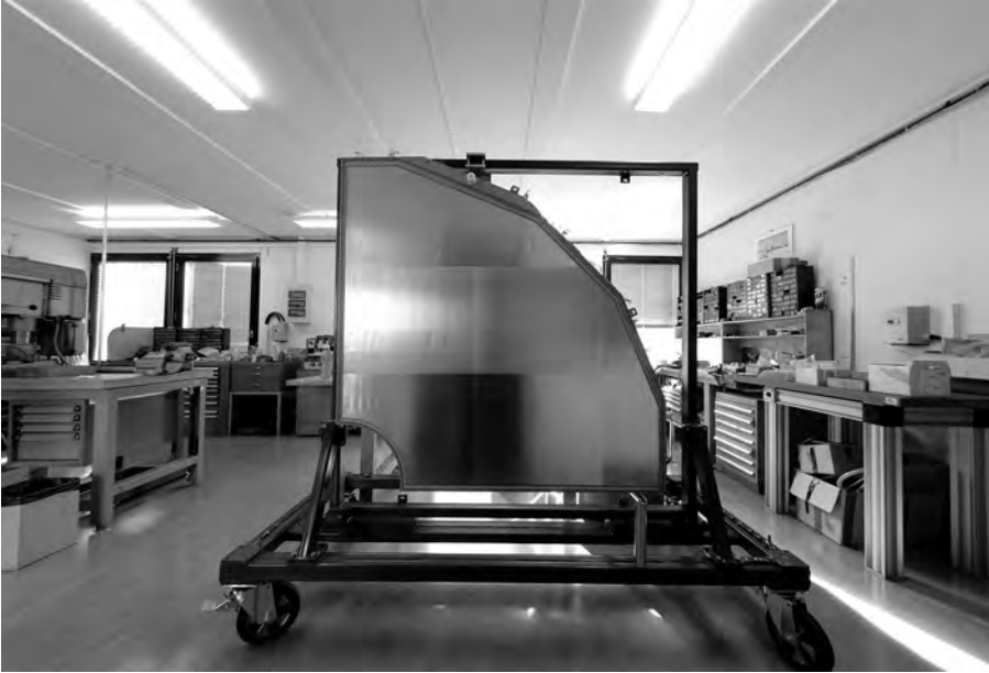
Figure 10.17 A segment of the ALICE TPC MWPC end-cap. Picture CERN (2002).
