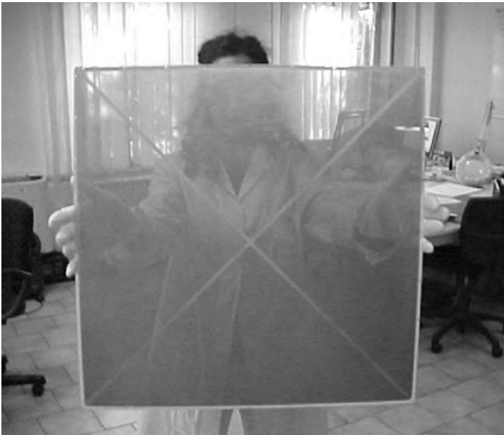
Figure 13.27 A prototype thick-GEM electrode developed for the COMPASS RICH upgrade (Alexeev et al. , 2010). By kind permission of Elsevier.
