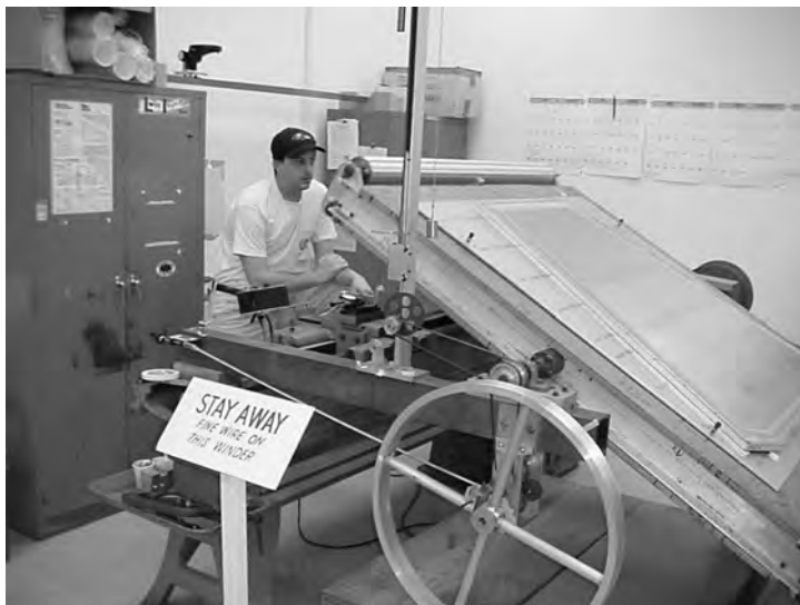
Figure 8.58 A rotating frame winding machine used for the wiring STAR TPC MWPC modules. Courtesy Brookhaven National Laboratory (USA).
