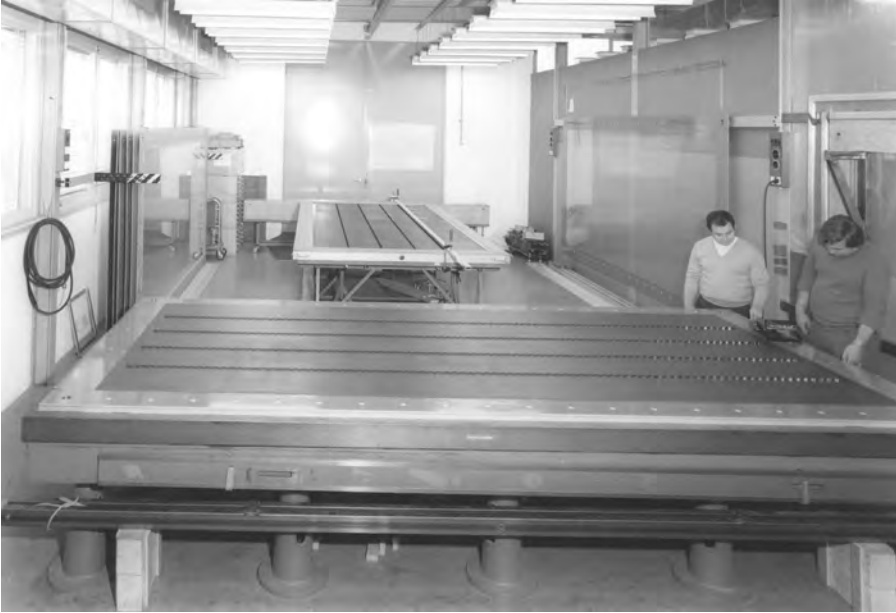
Figure 9.15 A wire plane of the large Omega drift chamber under construction. Picture CERN (1976).
