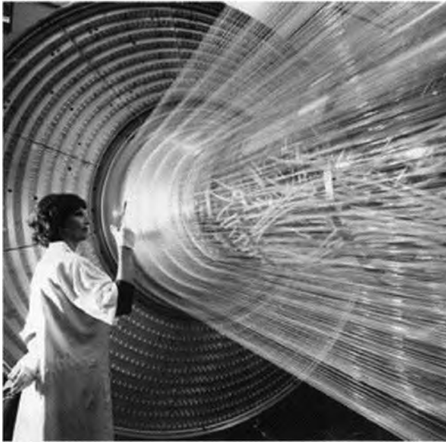
Figure 9.21 A cylindrical drift chamber in construction for the MARK II detector. Picture courtesy SLAC (1977).
