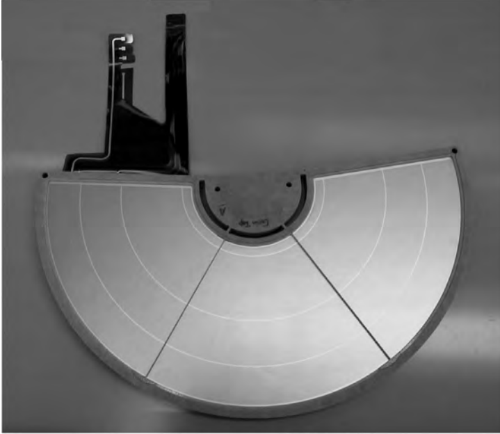
Figure 13.26 A semi-circular GEM electrode, 30 cm in diameter, for the TOTEM experiment. Picture CERN (2004).
