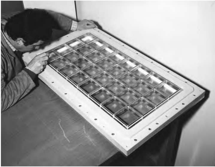
Figure 14.12 The large composite \text{CaF}_2 window of the E605 RICH. Picture CERN (1982).
