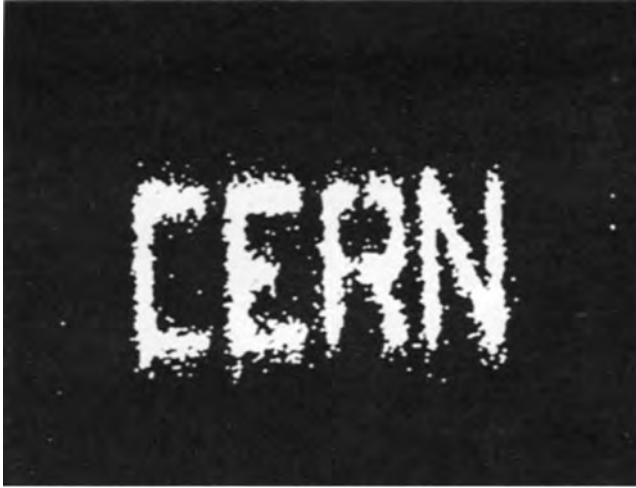
Figure 8.32 Two-dimensional X-ray image of a letter cut. The mask size is 4 \times 1.5 \text{ mm}^2 (Charpak et al. , 1978). By kind permission of Elsevier.
