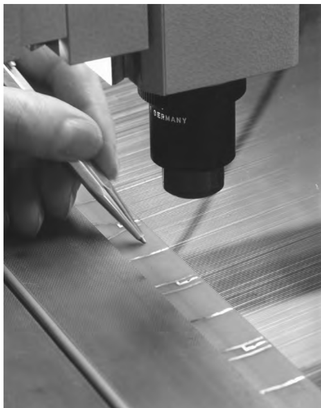
Figure 9.14 Close-up of the wire plane in the HADC. Picture CERN (1976).
