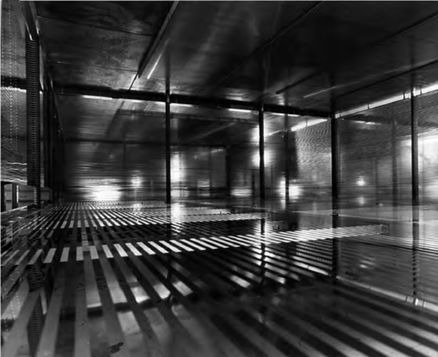
Figure 10.21 Inner view of one of the NA49 TPC modules. Picture CERN (1994).
