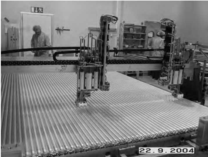
Figure 11.10 Construction and alignment of a MDT module. Picture CERN (2004).
