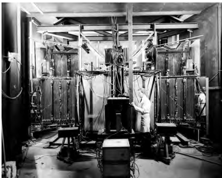
Figure 1.2 PS11, an optical spark chamber experiment at CERN's Proton Synchrotron, with accidental cosmic rays tracks. Picture CERN (1967).
