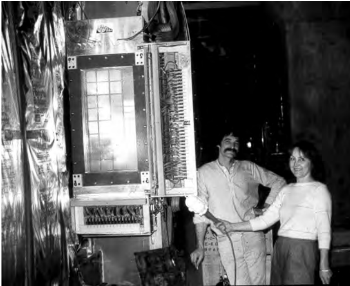
Figure 1.15 Philippe Mangeot and Anna Peisert with one of the photon detectors of the E605 RICH at Fermilab. Picture by the author (1980).
