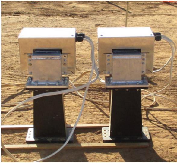
Figure 11.13: Prototype two horn antennae microwave system operated through two 2.45 GHz domestic microwave ovens (EMS8586V; Sanyo; Tokyo, Japan) used for soil irradiation in field conditions.
