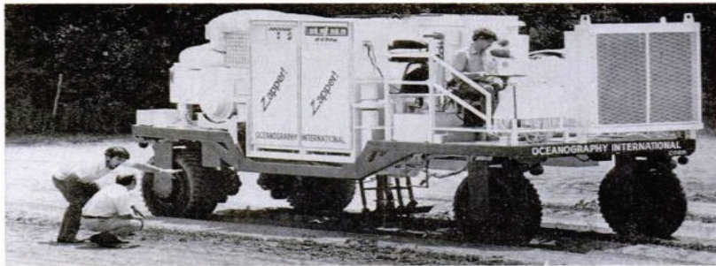
Zapper III zaps weed and soil pests by discharging high-powered microwaves into the ground via a sled-shaped emitter. Developed by Oceanography International Corp., Zapper can increase crop yields without the risk of pesticide use.
