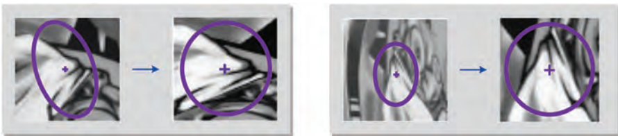
Figure 8.8 Affine-Invariant Interest Point Detection. The circular point neighborhood is replaced with an ellipse in order to achieve independent orthogonal varying detection scales for interest point detection. Before applying a detection algorithm, the local neighborhood is affine normalized, which results in a circular neighborhood and a transformed image patch (from [7]).
