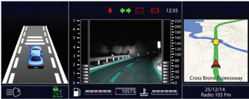
Figure 10.7 Holistic HMI layout with the night vision system in the central area.
