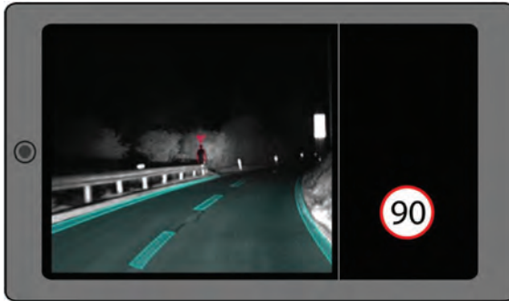
Figure 10.14 Smart HMI concept: Nomadic device with night vision system.
