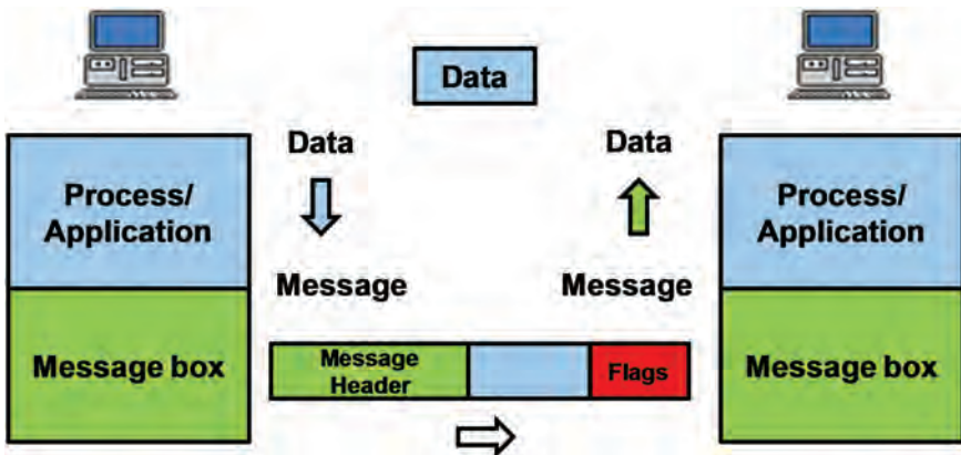
Figure 2.12 Message box principle for intra-unit communication.
