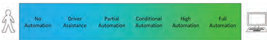
Figure 9.12 SAE J3016 standards of driving automation levels for on-road vehicles.
