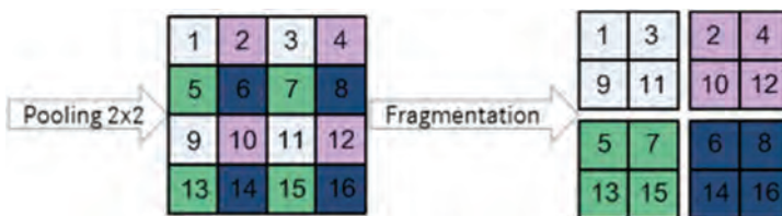
Figure 6.3 Example of a fragmentation after a 2 \times 2 pooling. The naïve approach would only produce the bright pixels, while an overlapping pooling produces all other possible pixels (purple, green, and blue). These pixels must be reordered to be able to correctly continue with the forward propagation of the neural network.
