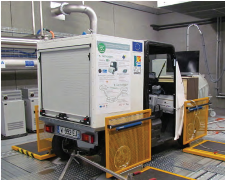
Figure 11.7 The Biocar test vehicle on the Horiba chassis dynamometer.
