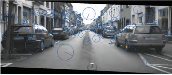
Figure 8.20 Comparison of the resulting SIFT-features of the left input image for 12 bpp images and 8 bpp images. In the 12 bpp input image, an overall number of 1,069 features have been detected, whereas in the 8 bpp input image 1,056 features have been determined. A subset of 1,045 features (97.8%) is identical in both images (blue). There are 14 (1.3%) exclusive 8 bpp feature positions (red) detected and 24 (2.2%) exclusive 12 bpp feature positions (orange).
