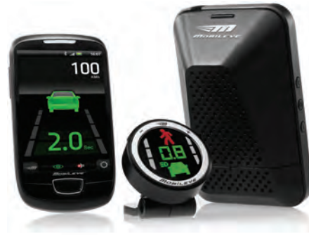
Figure 11.5 Mobileye 560 aftermarket vision-based ADAS.
