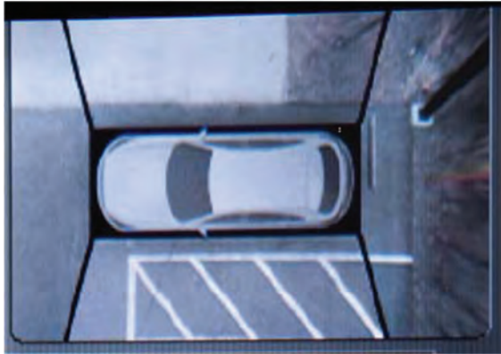
Figure 9.7 Top view of a parking assistance system.
