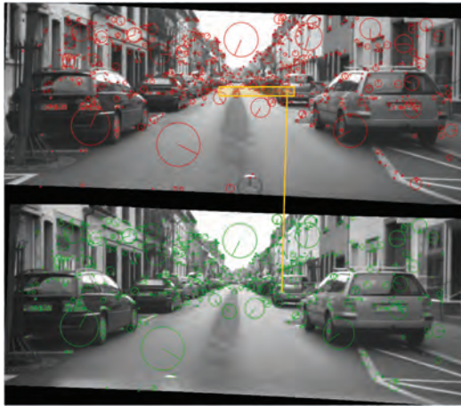
Figure 8.17 Extracted SIFT-features with exemplary geometry-based restriction of matching candidates. By restricting possible matching candidates geometrically, the problem size is significantly reduced.
