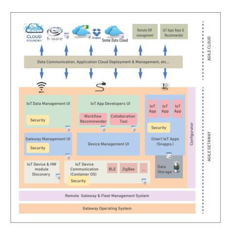
Figure 4.1. AGILE Detailed Architecture
