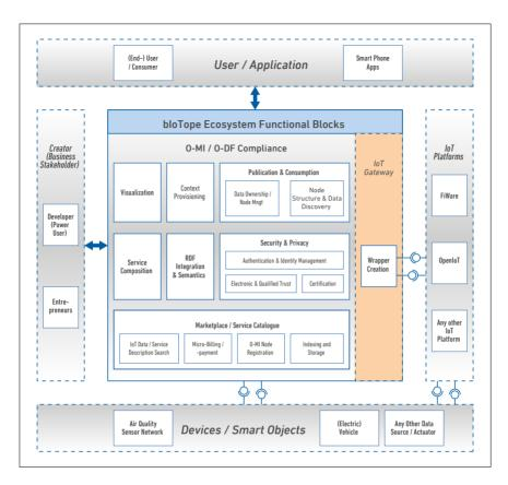
Figure 4.8. bloTope reference architecture.
