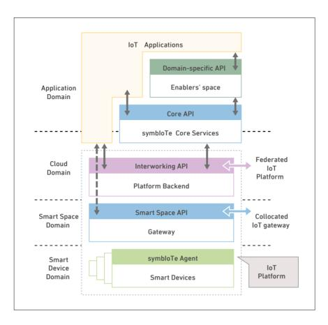
Figure 4.10. The symbloTe high-level architecture
