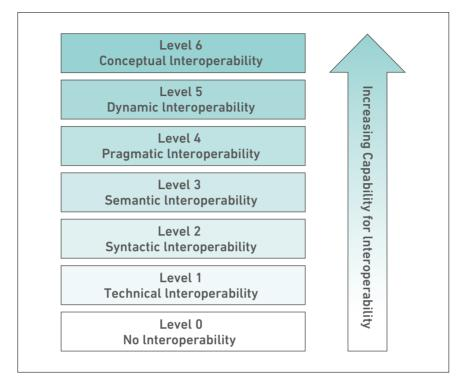
Figure 3.1. The Levels of Conceptual Interoperability Model [7].
