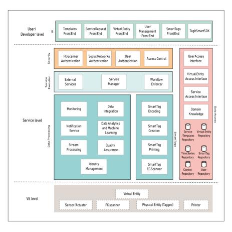
Figure 4.12. TagltSmart Platform Functional Architecture
