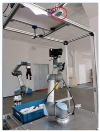
Figure 3.2.5 Setup for object 3D reconstruction.
