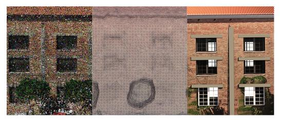
Dense point cloud (left), surface polygonal model (middle) and textured BIM model (right). (Author elaboration).
