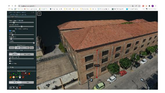
Fig. 05. Potree facilitates basic measurements on the rendered point cloud (author elaboration). However, the Potree renderer is only capable of displaying point clouds. In many application cases, for sharing with non-technical users, point clouds are treated as raw data, intended to be refined by conversion into triangular models (the meshes) or two-dimensional images. An important element of this study is to show the potential of the meshed model created, based on the obtained point cloud.
