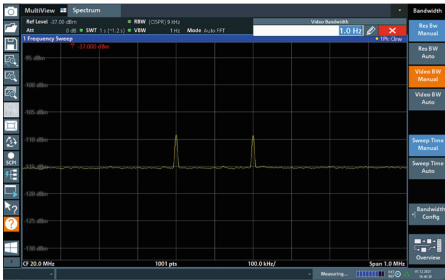
Fig. 6.11 Measurement of the same signal with different video bandwidths (VBWs). Measurements performed with R&S®FSV3013 by Rohde & Schwarz. (a) VBW = 200 kHz. (b) VBW = 1 Hz
