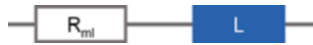
Fig. 11.24 Equivalent circuit of an inductor when considering magnetic losses only and ignoring ohmic losses and winding capacitance
