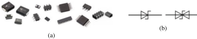
Fig. 11.43 TVS diodes. (a) Different form factors of TVS diodes. Courtesy of Würth Elektronik GmbH. (b) Left: unidirectional TVS diode. Right: bidirectional TVS diode
