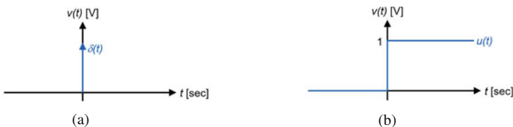
Fig. 15.2 Time-domain characterization functions. (a) Impulse Dirac delta function \delta(t) . (b) Unit step function u(t)
