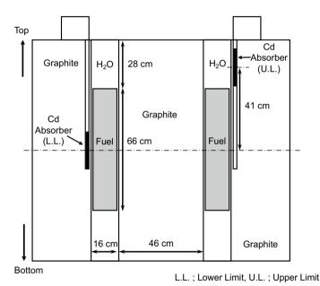
Fig. 2.4 Axial view of positional relationship between control rod (safety rod) and fuel plate in
