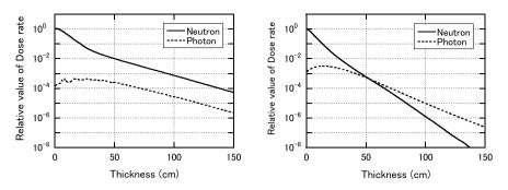
Fig. 3.17 Shielding against 1 MeV neutron radiation (left: graphite; right: concrete)
