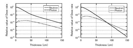
Fig. 3.18 Shielding against 2 MeV neutron radiation (left: graphite; right: concrete)
