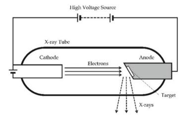
Fig. 3.27 Configuration of X-ray generator
