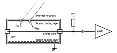
Fig. 5.8 Structure of boron-lined proportional counter
