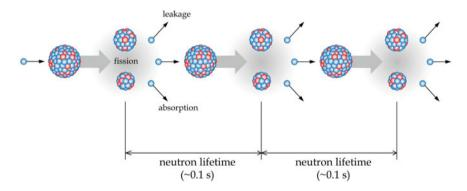
Fig. 1.12 Scheme of fission chain reactions
