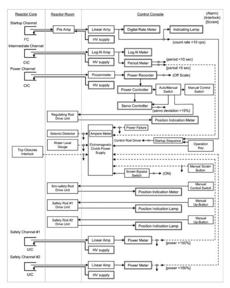
Fig. 5.11 Compositions of nuclear instrumentation of UTR-KINKI
