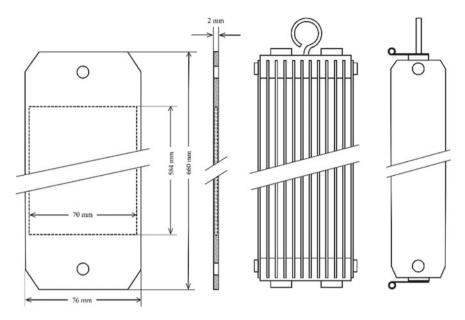
Fig. 1.6 Detail of fuel plate (left) and fuel assembly (right)
