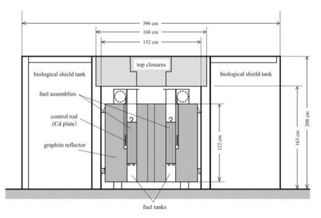
Fig. 1.4 Side view of UTR-KINKI reactor (North–South direction)
