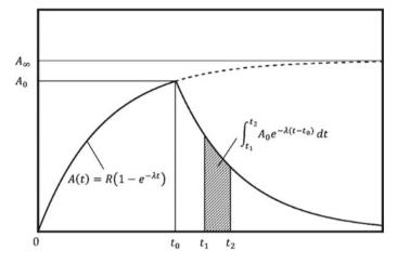
Fig. 3.7 Change in radioactivity of target material irradiated with neutrons for time  $t_0$
