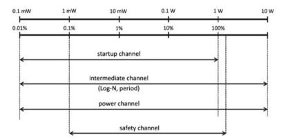
Fig. 5.10 Measurement power range of nuclear instrumentation of UTR-KINKI
