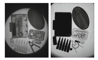
Fig. 3.29 Radiographic images of same objects using neutrons (left) and X-rays (right)
