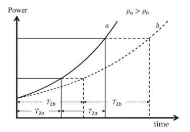
Fig. 2.5 Relationship between reactivity and reactor power
