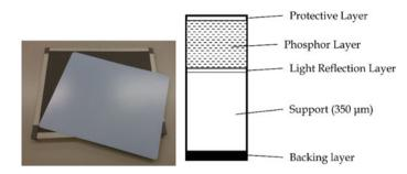
Fig. 3.24 IP (left) and cross-sectional structure (right)
