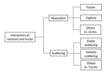
Fig. 1.10 Reactions between neutrons and nuclei
