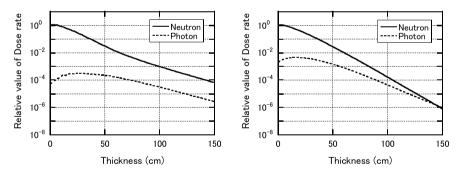
Fig. 3.19 Shielding against 3 MeV neutron radiation (left: graphite; right: concrete)
