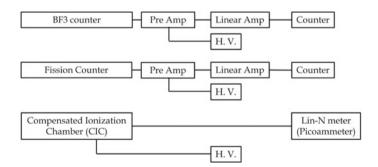
Fig. 2.2 Neutron measurement system used in approach to criticality experiment
