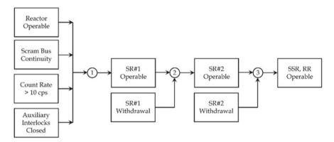
Fig. 1.18 Control rod withdrawal interlock circuit of UTR-KINKI
