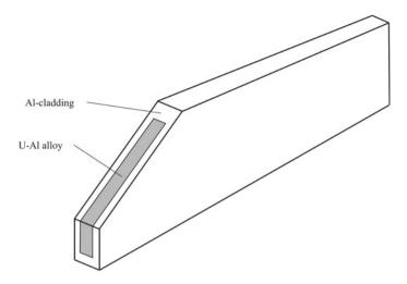
Fig. 1.5 Structure of the fuel plate
