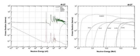
Fig. 3.1 Cross sections of Al-27 for neutrons (Data from Ref. [1])
