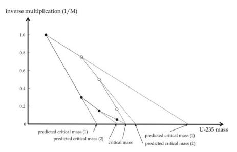
Fig. 2.1 Relationship between inverse multiplication 1/M and critical mass of U-235 fuel
