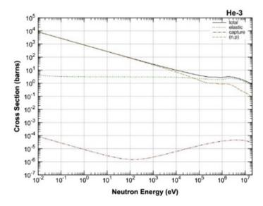
Fig. 3.14 Reaction cross section of He-3 (Data from Ref. [1])
