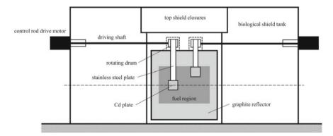
Fig. 1.8 Side view of operation of the Cd plate by control rod drive mechanism
