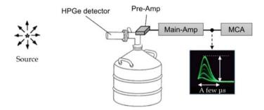
Fig. 3.21 Configuration of  $\gamma$ -ray spectrum measurement system
