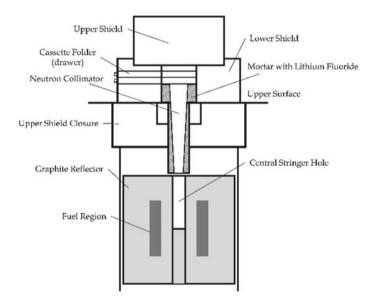
Fig. 3.26 Cross-sectional view of neutron radiography facility in UTR-KINKI
