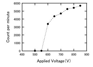
The voltage to be used is determined by obtaining the plateau curve of the GM counter while changing the applied voltage using a  $\beta$ -ray radiation source. Figure 3.5 shows an example of the plateau curve. The working voltage should be set at about 1/3 of the plateau length from the counting start voltage, which is 700 V, as shown Fig. 3.5.
