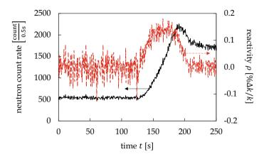
Fig. 2.9 Example of reactivity estimation using inverse kinetics method
