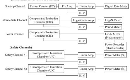
(Instrumentation & Control Channels)
