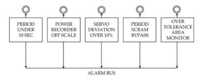
Fig. 1.16 Alarm circuit of UTR-KINKI
