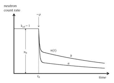
Fig. 2.7 Relationship between reactivity and output change by rod drop method
