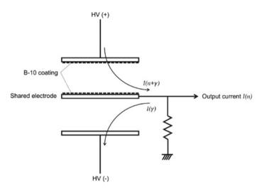
Fig. 5.9 Operation principle of compensated ionization chamber (CIC)
