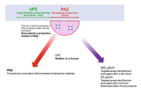
**Fig. 6.4** Concept of off-site evacuation based on nuclear emergency response guidelines (Ref. [4]) (Translated under the creative commons attribution license 4.0 (https://creativecommons.org/lic enses/by/4.0/) from [4] Copyright agency for natural resources and energy)
