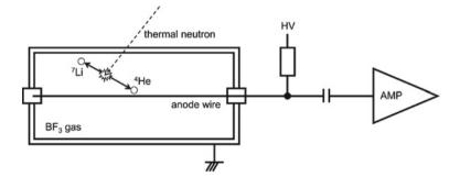
Fig. 5.2 Structure of BF<sub>3</sub> proportional counter
