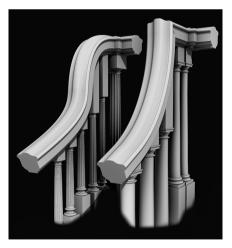
**Figure 11.2:** Staircase construction, swan-neck ramp (left) and concave ramp (right).
