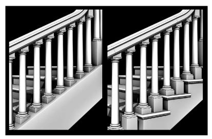
**Figure 11.1:** Staircase construction, closed string (left) and open string (right).
