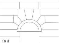
**Figure 7.16:** (a–d) Alternative possible rusticated patterns around niche heads of the Printing House: 16a with seven voussoirs; 16b with shallower horizontal courses; 16c with springing of arch aligned with a horizontal course; 16d as executed, lacking the infelicities of 16a–c. Drawings by the author.
