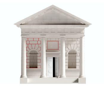
**Figure 7.15:** Printing House, Trinity College Dublin, elevation showing relationship of columns to inner wall of portico.
