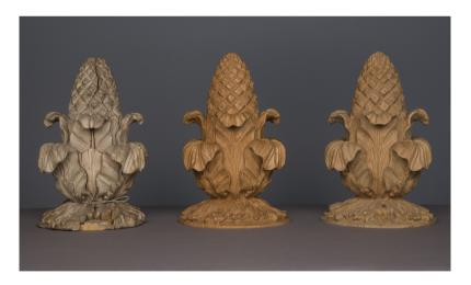
**Figure 2.32:** Original Cassiobury staircase finial (left), milled replica finial with hand-carved and sealed surface (centre), completed replica finial (right).
