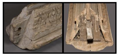
**Figure 2.28:** Handrails from Cassiobury (left) and Eyrecourt staircases (right), showing the effects of the chemical stripping. Photographs © The Metropolitan Museum of Art and Mechthild Baumeister.
