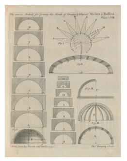
**Figure 5.10:** Plate LVIII, 'The Various methods for forming the heads of circular & Elliptical Niches', Batty Langley, *The City and Country Builder's and Workman's Treasury of Designs*. London: Printed and Sold by S. Harding, 1745.
