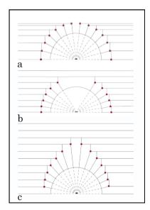
**Figure 7.6:** (a) A semicircular 'halo' can be associated with courses of unequal height; (b) a semicircular 'halo' can be associated with voussoirs and keystone of disproportionate sizes; (c) a raised 'halo' with voussoirs leading continuously into rusticated courses of equal height. Drawings by the author.
