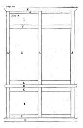
**Figure 10.8:** Joseph Moxon, *Mechanick Exercises*. Midwinter and Leigh, London, 1703, p. 102, Plate 7. 'AAA=The Stiles B=The Base C=The Lower Rail D=The Sur-Base EE=The Middle Rail or Rails F=The Friese [sic] Rail G=The Upper Rail H=The Cornice I=The Lying Pannel K=The Large Pannel L=The Friese Pannel'.
