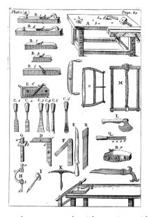
**Figure 10.16:** Joseph Moxon, *Mechanick Exercises*. Midwinter and Leigh, London, 1703, p. 102, Plate 7. Caption: C.1 = former C.2 = paring chisel, which 'must have a very fine and smooth edge: its Office is to follow the Former, and to pare off and smoothen the irregularities the former made'. HathiTrust.
