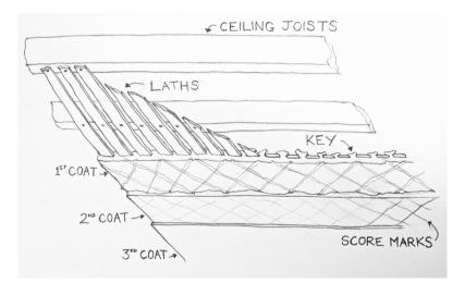
**Figure 9.2:** Diagram of three-coat plaster.
