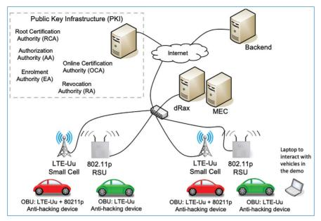
Figure 28. Global components of the testbed for attack on V2X message transmission.
