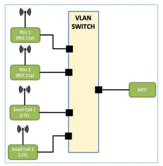
Figure 3. Connection of radiating infrastructure to the MEC.
