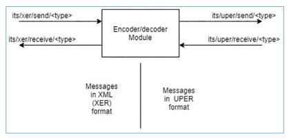
Figure 10. The Encoder/Decoder module with an example of MQTT queue's names.
