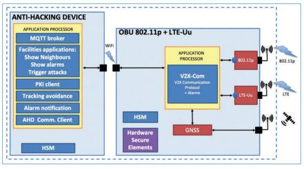
Figure 2. OBU and anti-hacking device components.
