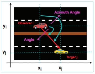
Figure 6. Angle and azimuth angle measurement.
