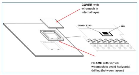
Figure 27. Illustration of GNSS metal lid protection.
