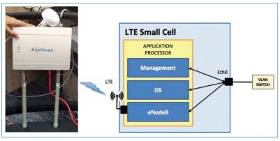
Figure 7. LTE small cell plus its components.
