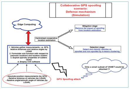
Figure 7. High-level architecture of collaborating defence mechanism.
