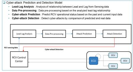
Figure 8. RCV cyber-attack prediction and detection model.
