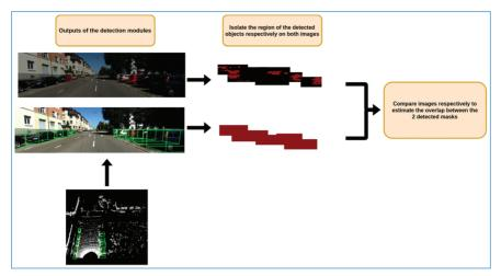
**Figure 20.** Comparison scheme. The 3D isolated projected objects are compared respectively with the segmentation output.
