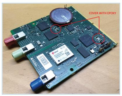
Figure 22. Clock oscillators covered with epoxy.
