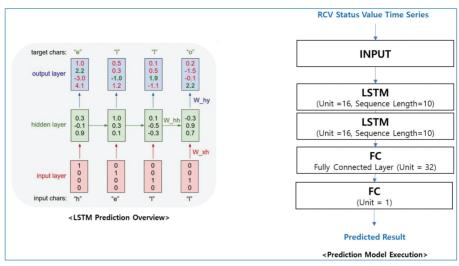
Figure 9. LSTM Execution Overview for RCV Cyber-attack Detection.
