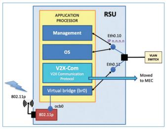
Figure 4. IEEE 802.11p RSU components.
