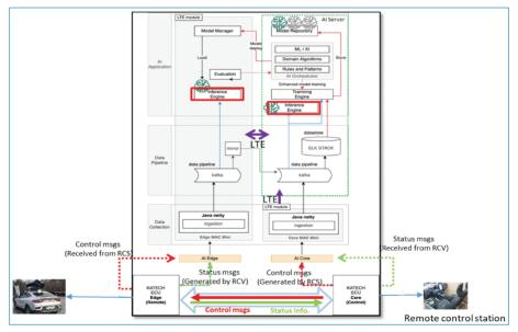
Figure 6. RCV threat detection and prediction functional architecture.
