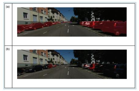
**Figure 18.** Image (a) is the output of the segmentation model to the non-attacked image while in the image (b) is the output of the segmentation model to the attacked image. The red mask indicates the detected vehicles.
