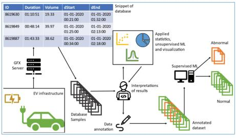
Figure 6. Semi-supervised Machine-Learning pipeline.
