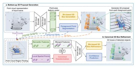
**Figure 17.** [18] The PointRCNN architecture for 3D object detection from point clouds. The whole network consists of two parts: (a) for generating 3D proposals from raw point cloud in a bottom-up manner, (b) for refining the 3D proposals in canonical coordinates.
