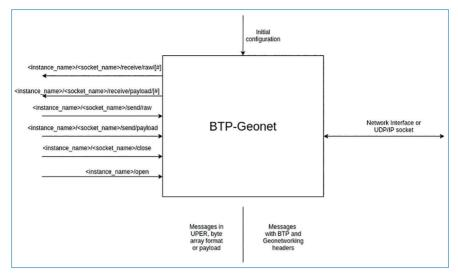
Figure 11. The BTP/Geonet module with an example of queues names.
