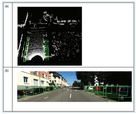
**Figure 19.** (a) The output of PointRCNN to 3D space in the LiDAR coordinate system. (b) The projected output of PointRCNN to the image plane.
