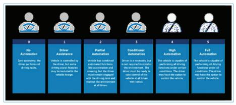
Figure 1. Society of automotive engineers (SAE) automation levels.
