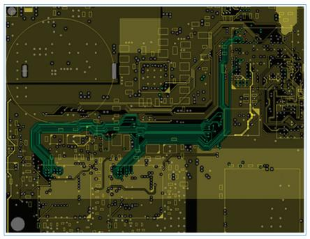
Figure 24. Secure signals between microprocessor and V2X transceiver.
