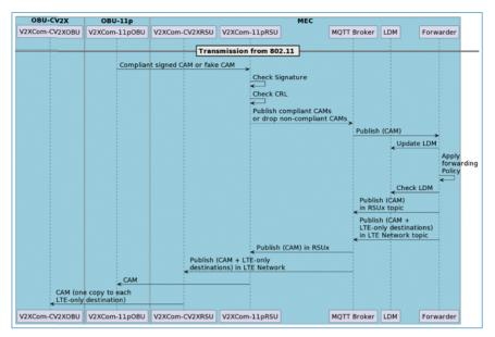
**Figure 30.** Workflow of use case "Interoperability between different radio technologies" when the transmission is initiated from a vehicle provided with 802.11p and LTE-Uu interfaces.
