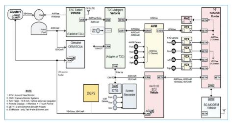
Figure 2. Overall architecture of sensor system of test vehicle.
