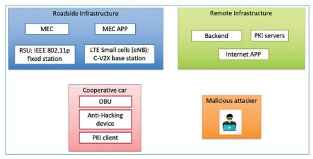
Figure 1. Global components of V2X system.
