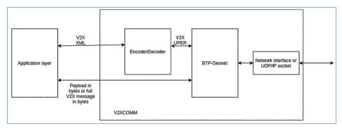
**Figure 9.** General architecture of an application or set of applications using the V2XCOMM module.
