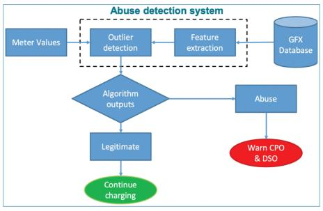
Figure 5. An overview of the Abuse Detection workflow.
