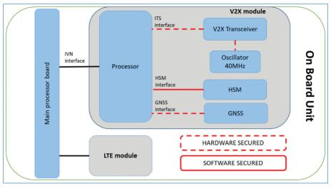
Figure 18. High level scheme of OBU system blocks.
