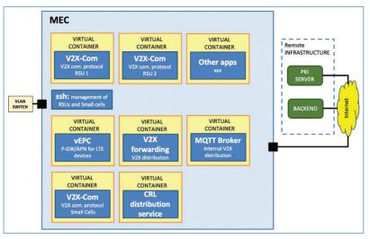
Figure 8. MEC components.
