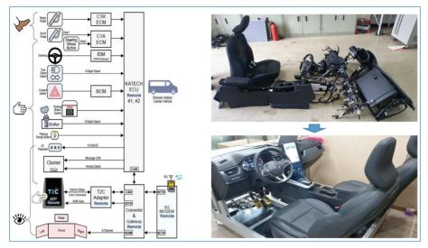
**Figure 5.** System architecture of the remote control station (left) and implementation of the remote control station (right).
