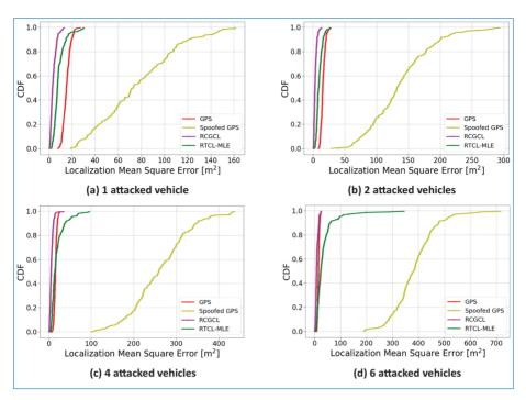
**Figure 9.** CDFs of LMSE of the proposed cooperative and robust schemes for different number of compromised vehicles.
