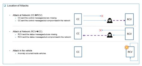
Figure 7. RCV cyber-attack scenarios.
