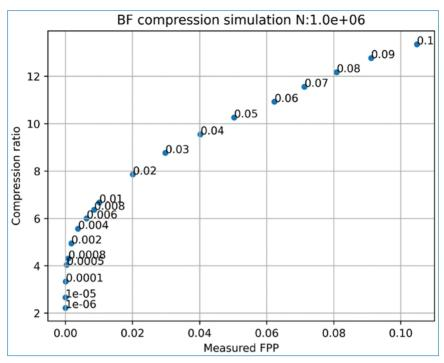
Figure 15. Compression gain against simulated (measured) false positive rate.
