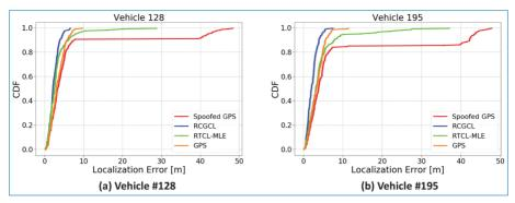
Figure 12. Localization Error of spoofed vehicles.
