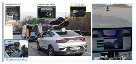
**Figure 11.** Field trial of the remote controlled vehicle use case via mmWAVE communication in KATECH testing ground.
