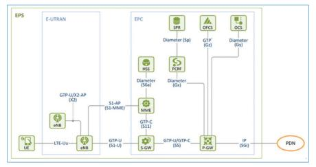
Figure 6. LTE network architecture.
