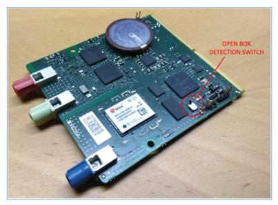
Figure 21. Open box detection switch.
