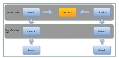
Figure 15. Abstract sensor fusion architecture describes where the late fusion occurs.
