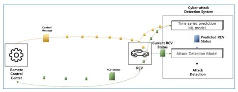
Figure 10. Overview of RCV cyber-attack detection solution.
