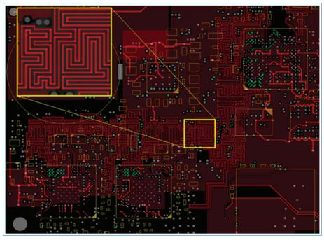
Figure 25. Wire-mesh used to cover secure signals from top layer.
