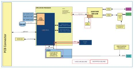
Figure 19. V2X module hardware blocks.
