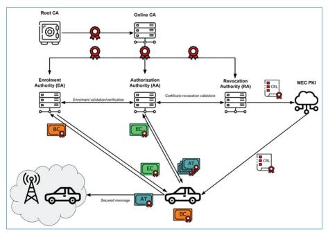
Figure 14. PKI-Toolbox high level architecture.
