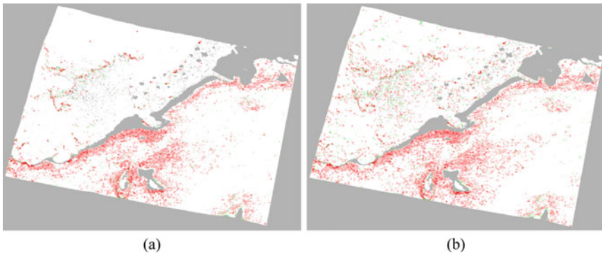
Fig. 5.13 Point cloud coloured according to the distance to the surface. White points are closer than 0.4 m, green points lie below the surface and red points above. More saturated colour means larger distance. The size of the white points are reduced compared to the coloured points. a Tolerance 0.1 m, 12 iterations, b tolerance 0.6 m, 12 iterations
