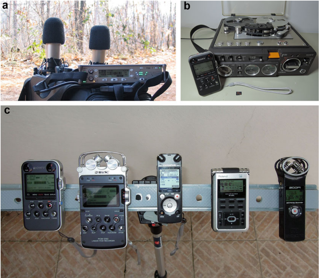
Fig. 1.9 (a) Photograph of a professional portable high-quality recorder (Sound Devices, SD722) with both hard disc and solid-state memory recording capabilities, connected to two low noise microphones (Rode NT1A) for soundscape recording. (b) Photograph of SONY TC-510 open-reel recorder (1982) and a SONY PCM-M10 digital recorder with its microSD memory
