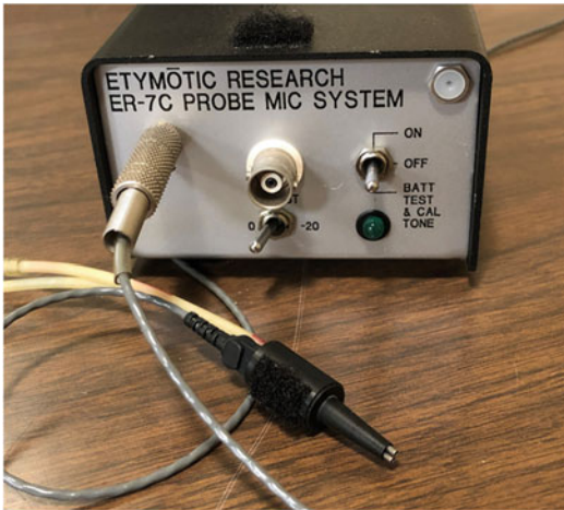
Fig. 10.14 A commercially available low-noise microphone with two external sound sources. The probe tip containing the microphone and sound tubes is covered with a foam or plastic ear tip and inserted into the ear canal to form a closed acoustic system. For animals without ear canals, the probe can be inserted into a plastic tube that is then sealed in place against the ear of the animal
