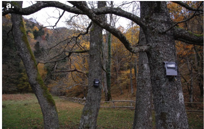
Fig. 2.19 (a) Photograph of autonomous acoustic recorders placed in the Sassofratino Nature Reserve, Italy. In the foreground, a Wildlife Acoustics Song Meter SM3. In the background, a custom recorder developed at the University of Pavia. (b) Wildlife Acoustics Song Meter SM4BAT-FS. (c) Titley Scientific Anabat Express. Permission to reprint by the respective manufacturers
