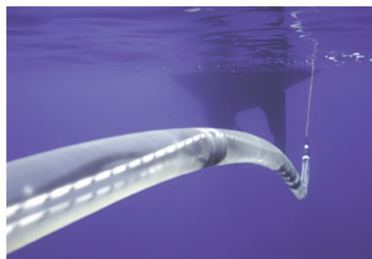
Fig. 2.15 Photograph of a towed array under water, developed by the University of Pavia (Italy), with the tow vessel in the background
