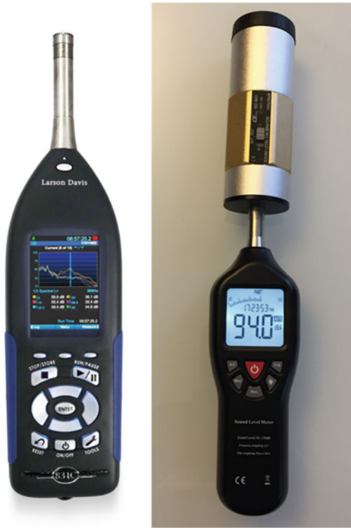
Fig. 2.29 Photograph of Larson Davis SoundAdvisor 831C sound level meter with spectral analysis and sound recording capabilities (left; permission to reprint from Larson Davis ( http://www.larsondavis.com/ ; accessed 5 Mar. 2021)) and of a simple noise-level analyzer with calibrator (right; shown being calibrated using a 1 kHz tone with 94 dB SPL)
