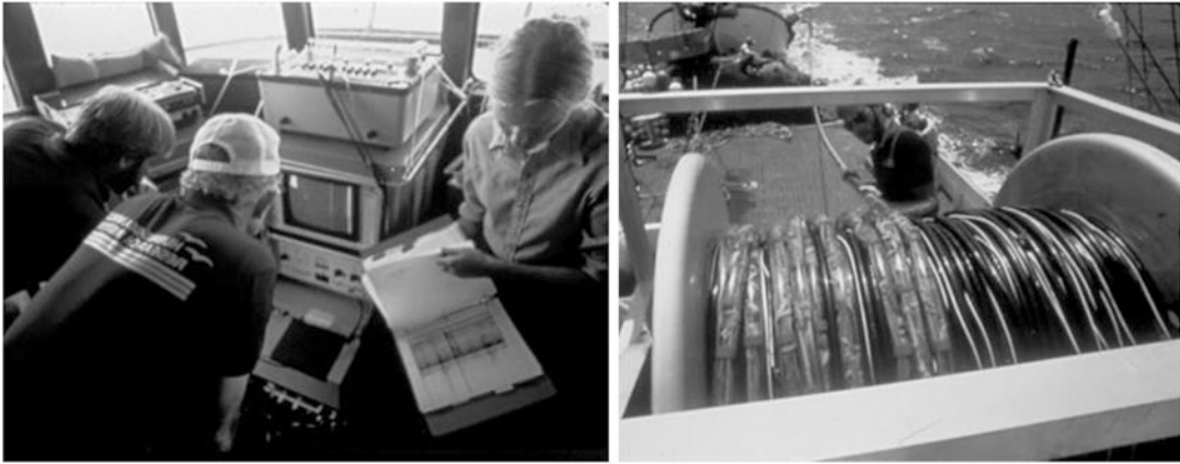
Fig. 1.18 Left: Photograph of the topside electronics required to receive, record, and process data from a towed array in 1983. Right: Photograph of deploying a towed array from the deck of a tuna seiner, the MV Queen
