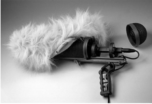
Fig. 2.9 Photograph of a microphone setup with pistol grip and elastic suspension, foam windsock, and additional furry windsock for maximum wind protection. Reprinted with permission from Sennheiser
