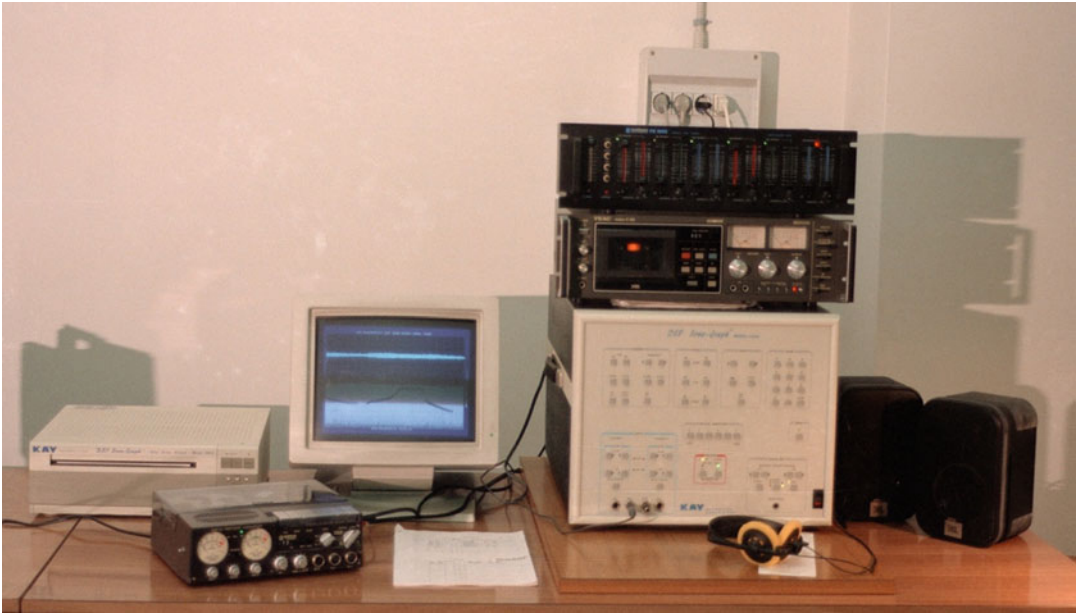
Fig. 1.26 Photograph of the University of Pavia bioacoustic laboratory equipment in 1989 with a Kay Sona-Graph DSP 5500, color monitor, thermal printer,
