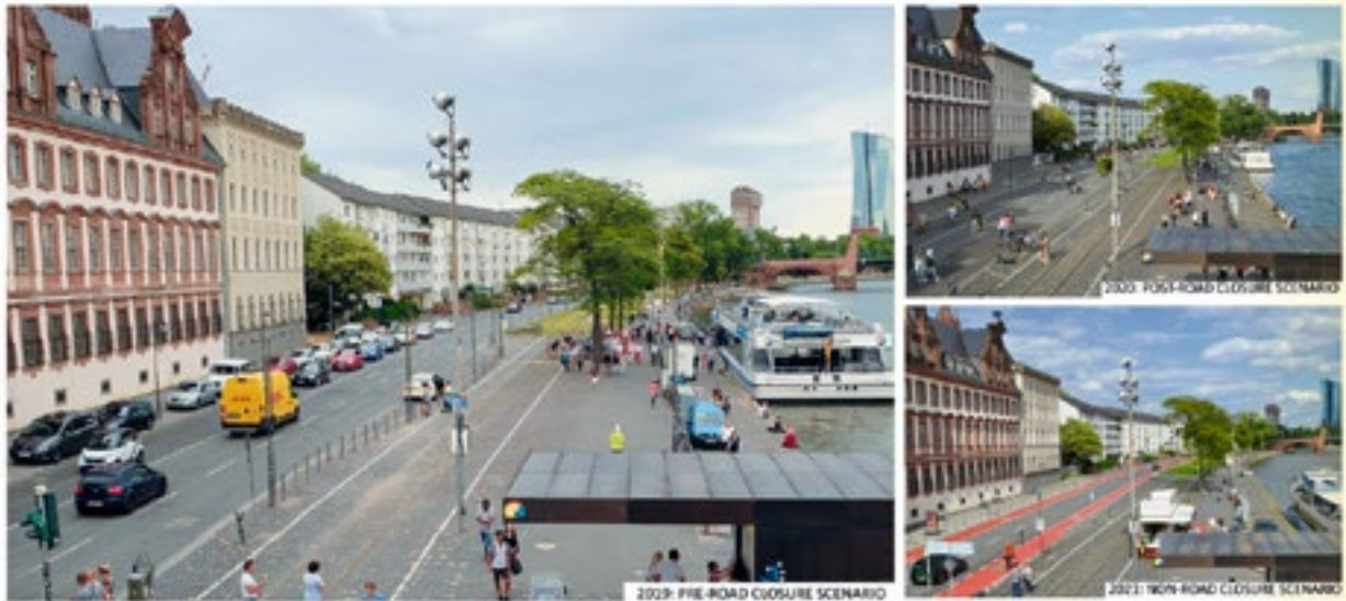
Fig. 1 Mainkai street before, during, and after road closure in 2019, 2020, and 2021, respectively. Note: The cycle lanes in 2021 were painted permanently after data supported the initial recommendations presented to the Traffic Planning Department of Frankfurt am Main. (Source: Urban Design and Planning Unit, Technical University of Darmstadt)
