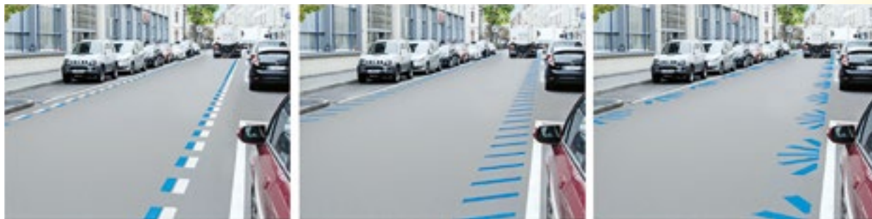
Fig. 4 Design variants for the demarcated door zone: the double dotted lines of the test route, diagonal hatching lines, and fanned-out lines (Source: Janina Albrecht; see Albrecht and Eckart 2020: p. 47)
