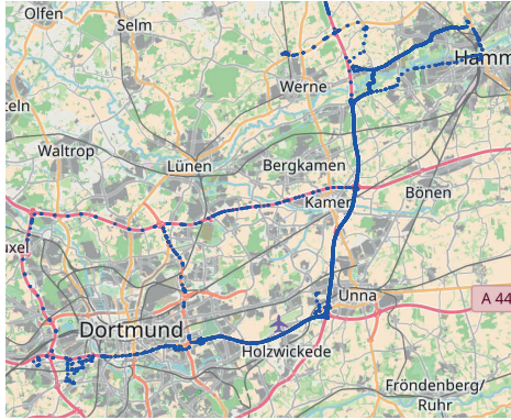
Fig. 9.16: Road map with locations of all data samples of the measurement campaign between two larger cities in Germany. Each blue point represents an intermediate status logging of all measured variables (cf. Table 9.3) during ongoing uplink transmissions. (Map: ©OpenStreetMap contributors, CC BY-SA). ©[2018] IEEE. Reprinted, with permission, from [207].
