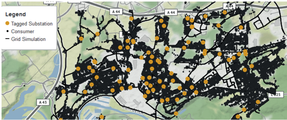
Fig. 5.4: Grid simulation and known substation locations in OSM for Witten. The road network contains 37 287 edges and 36 844 nodes, N = 35\,713 consumer and m = 1130 possible places for substations. The location of 127 substations is documented in OSM, but very likely several are missing, especially in the east.
