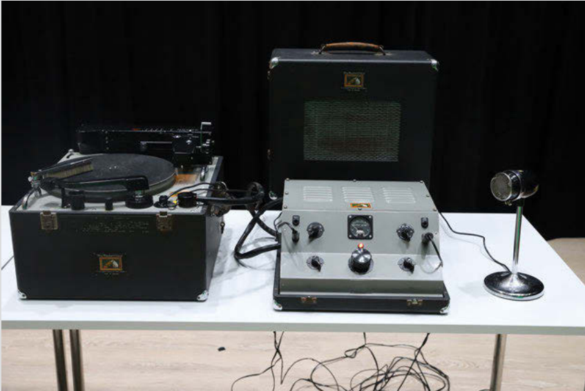
Fig. 6: The HMV 2300H: recording unit, amplifier, loudspeaker and microphone. Photo by Aleksander Kolkowski. Courtesy of the C 2 DH / University of Luxembourg.
