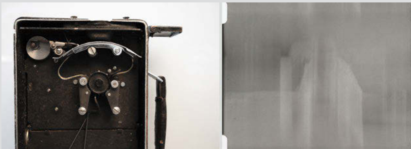
Fig. 35: White line indicator in the 16mm film camera and still from the distorted film. Photo by Tim van der Heijden. Courtesy of the C 2 DH / University of Luxembourg.
