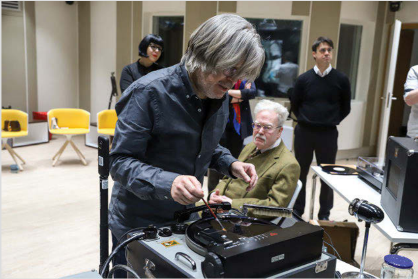
Fig. 9: Cutting a record on the HMV 2300H Portable Disc Recorder. Courtesy of the C 2 DH / University of Luxembourg.
