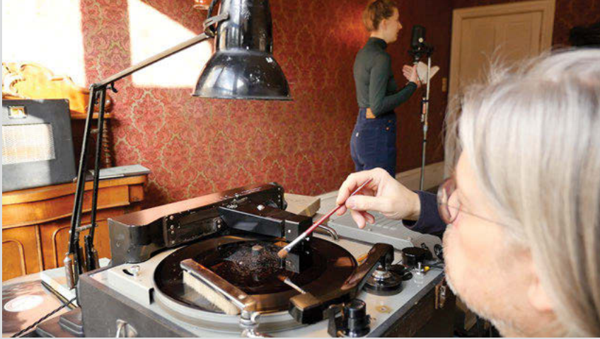
Fig. 33: Judith Westerveld making a recording on the HMV 2300H. Courtesy of Tijs de Bie.
