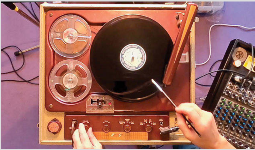
Fig. 7: Wilcox-Gay Recordio: recording from tape to disc. Photo by Aleksander Kolkowski. Courtesy of the C 2 DH / University of Luxembourg.
