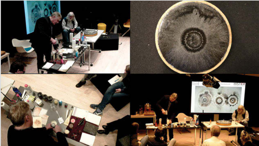
Fig. 37: Illustration of a Lichtenberg figure on a resin plate and its production, demonstrated by historians of science Falk Rieß and Wolfgang Engels. Courtesy of the C 2 DH / University of Luxembourg.
