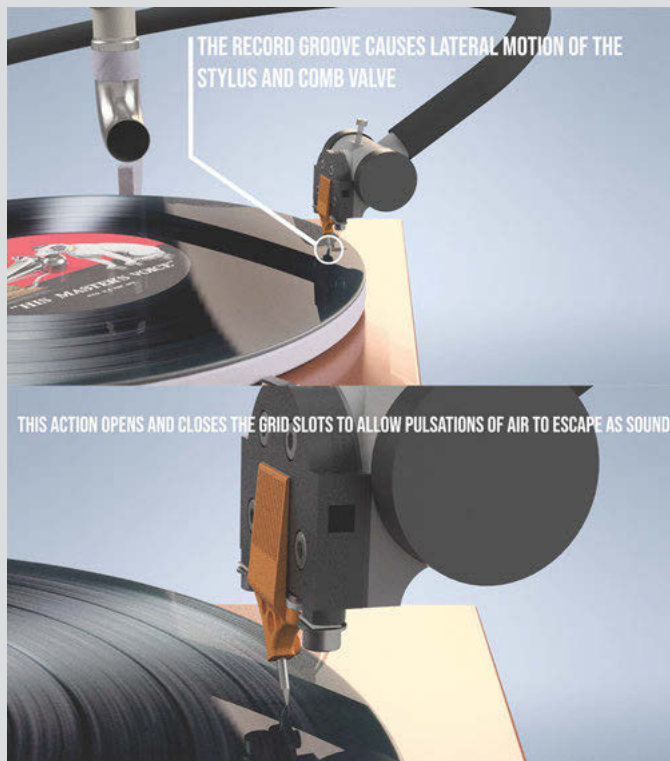
Fig. 61: Working function of a Stentorphone soundbox. Stills from animation by Thomas Theisen. Courtesy of the DoE / C 2 DH / University of Luxembourg.
