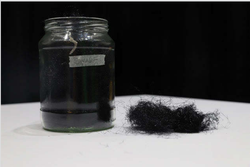
Fig. 45: Swarf from cutting records on the HMV 2300H. Photo by Aleksander Kolkowski. Courtesy of the C 2 DH / University of Luxembourg.
