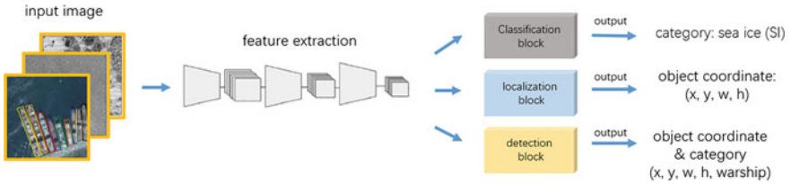
Fig. 21 Overview of a neural network-based recognition task. It contains the three basic computer vision tasks of classification localization and detection
