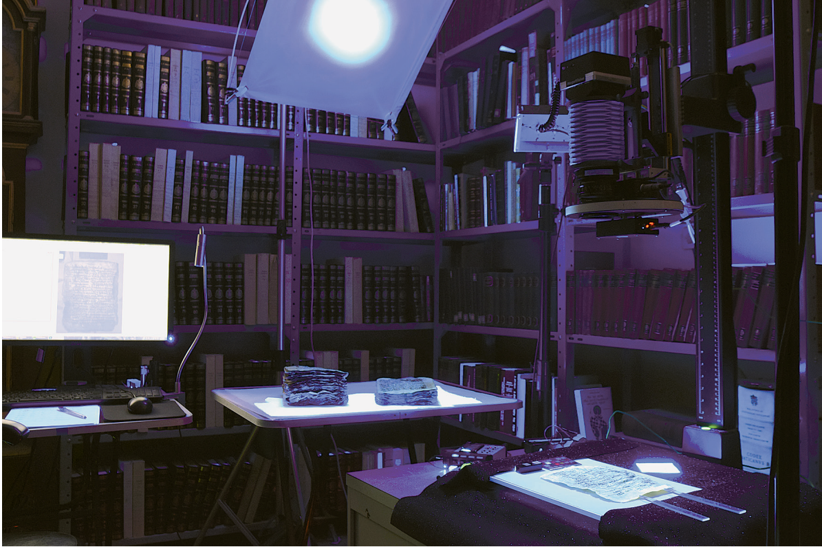
Figure 3 – Copy-stand used for imaging unbound folia and fragments in the foreground; computer for capturing data on the left (© Damianos Kasotakis, 2015)
