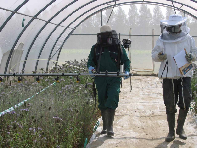
Figure 6 Application in a semi-field (tunnel) test with honey bees in phacelia according to EPPO 170.
