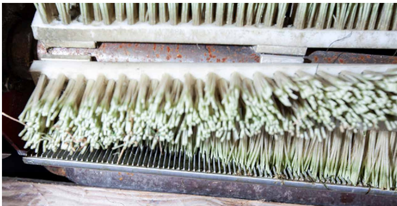
Figure 3 Bristles of the coarse brush interacting with the grooved baseblade of the Weedbine. Source: Henderson (2021).
