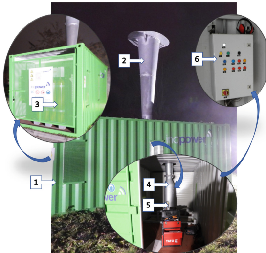
Fig. 2. Shock wave generator. 1 - Container, 2 - Outlet tube, 3 - Bundle of acetylene cylinders, 4 - Combustion chamber, 5 - Fuel inlet ports, 6 - Control cabinet.
