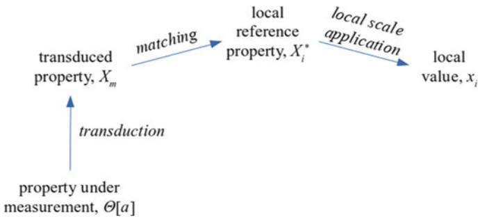
**Fig. 7.6** The first three stages of direct measurement: after transduction and matching, local scale application (in the example  $X_i^*$  is the position of the  $i$ -th mark etched on the scale of the thermometer and  $x_i$  is a value of position)
