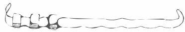
FIG. 46. A simple rack of bent wire suitable for the block-testing outlined in this study.
