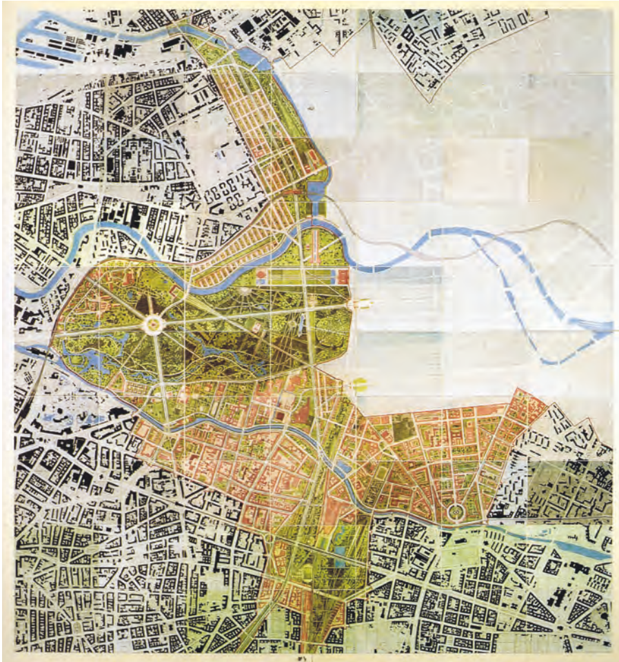
FIGURE 5 Masterplan Berlin 1984: the first overall urban development plan which points beyond the International Building Exhibition 1984/87 to possibilities of longer-term urban interventions. Plan made by 70 sheets, original drawing scale 1:5000
