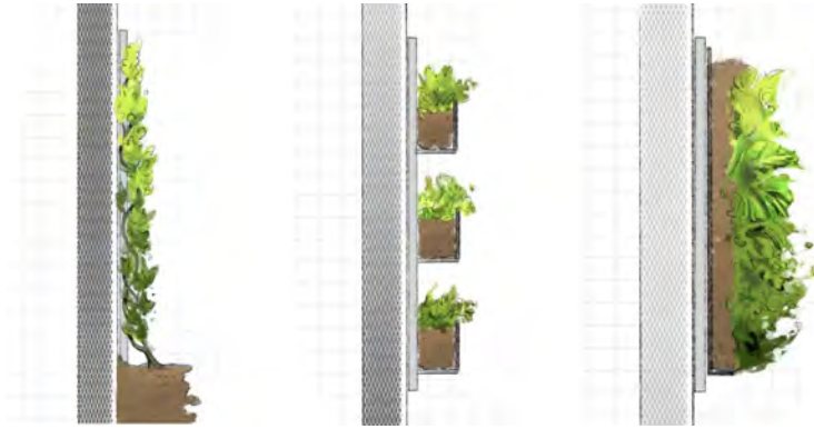
Figure I.1: Ground-based (left), pot-based (middle) and wall-based (right) green facade (image by Bibi Erjavec)
