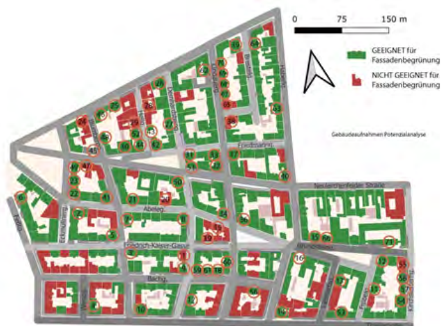
Figure III.12: Buildings suitable for VGS (green) and unsuitable for VGS (red) in the Deinhardstein-Grätzel (Vienna) (image by Samuel Schnöll)
