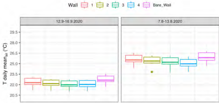
Figure IV.19: Mean daily temperature measurement for each individual wall as a boxplot for consecutive days with a maximum temperature over 30 °C for August and September 2020
