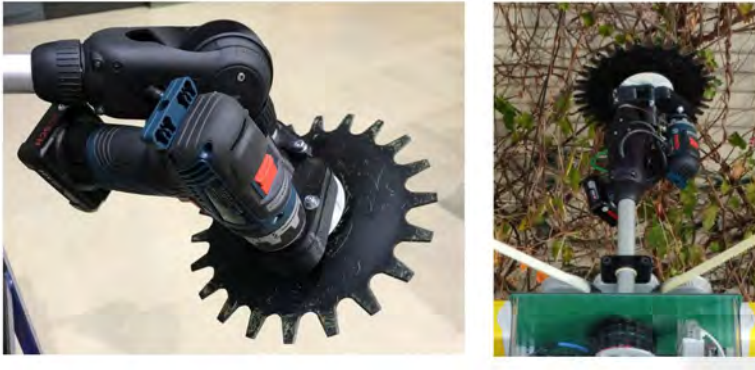
Figure III.23: Modified rotary scissor tool head for cutting thin branches and leaves (images by Sebastian Schröder)
