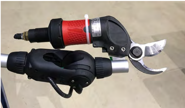
Figure III.24: Pruning shear installed at the robot (image by Sebastian Schröder)
