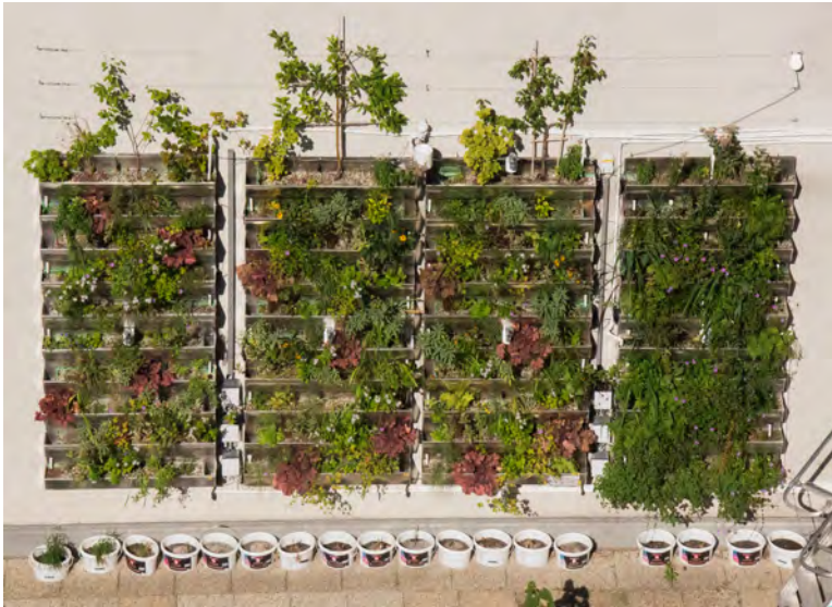
Figure III.7: Test wall at BOKU (from left to right): low irrigation once a week (scenario b), daily watering (scenario a) with tap water, daily watering (scenario a) with greywater, hourly watering (scenario c) for greywater treatment) (image by Irene Zluwa)
