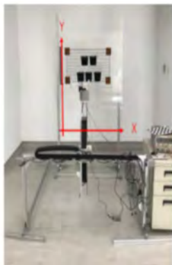
Figure III.21: Setup of the vertical green wall and gantry mechanism (image by Chung-Kee Yeh)
