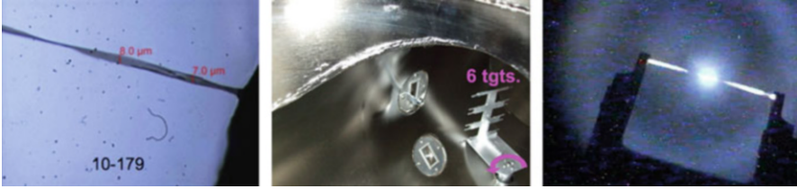
Fig. 12.8 Left: A carbon ribbon target. Center: Frame in scattering chamber holding six target. The frame rotates as shown by the arrow, sweeping the targets across the beam. Right: A target in the beam
