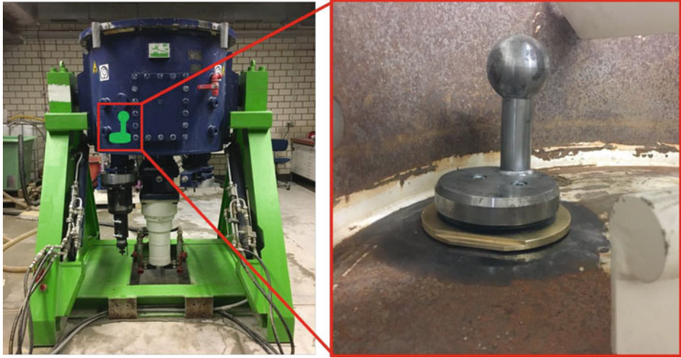
Fig. 4.9 COSMA large-scale test stand and installation position of the ball rheometer [36]
