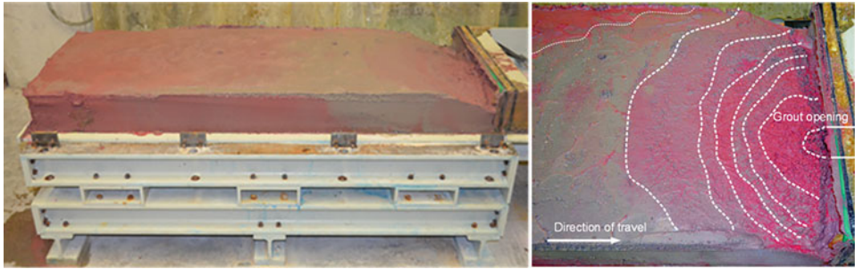
Fig. 5.45 Pressed one-component grout (left). Flow behavior of the grout (right) [70]
