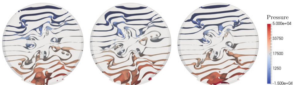
Fig. 4.42 Pressure contours in the chamber at 25 s, 27 s and 29 s, from left to right [25]
