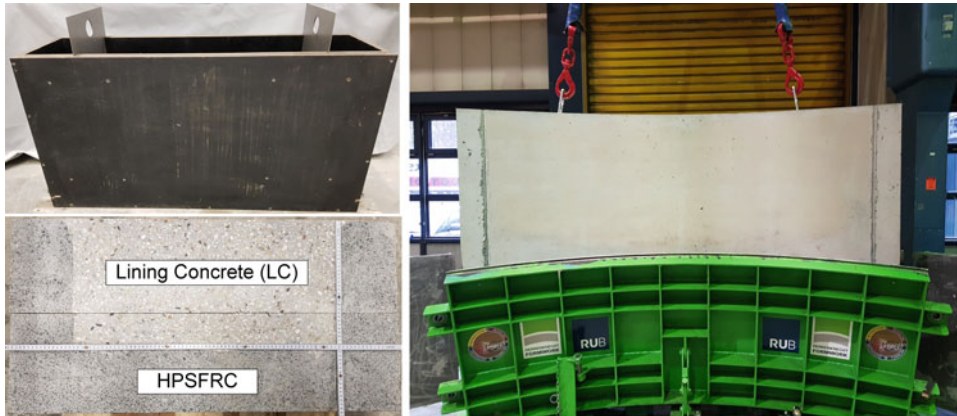
Fig. 5.17 Standing wooden formwork for the “wet-on-wet” production of hybrid specimens (top left), cutting surface through a hybrid specimen (bottom left) and standing segment formwork for the “wet-on-wet” production of hybrid lining segments in real scale (right)
