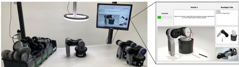
Fig. 4 Assembly stations equipped with graphical user interface and machine vision quality gate.
