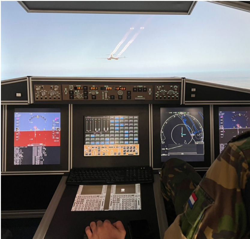
Fig. 9.3. Simulation environment used for the evaluation of the intercept guidance concept in March 2022. The picture was taken at the moment the intercepting aircraft had reached the desired position behind the TU-160 Blackjack.
