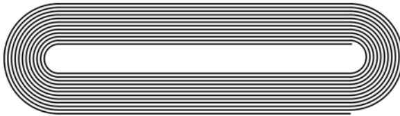
Figure 1.29. Racetrack coil wound with one tape. The turns are electrically isolated, with the current entering at one end of the coil and coming out at the other end.
