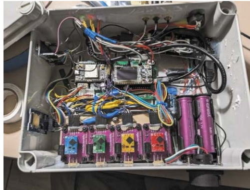
Figure 4 – The acquisition and transmission box. Measurements can be read in real time from the LCD display and are sent via mobile telephone and LoRa connectivity.
