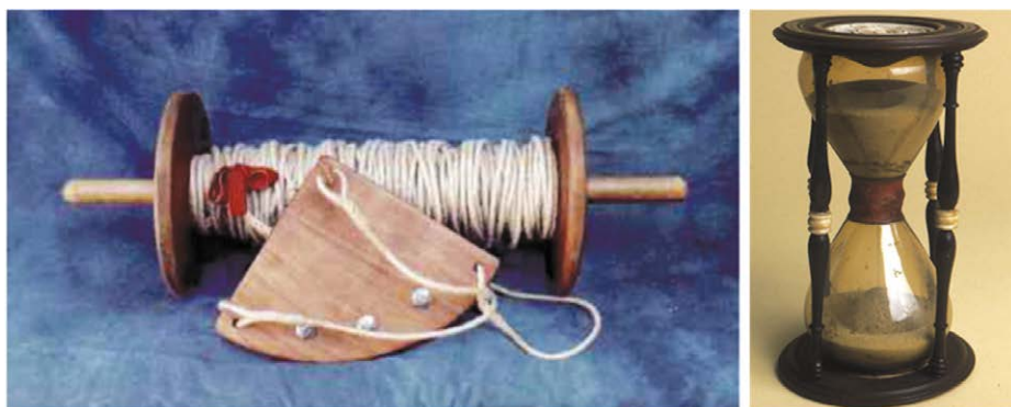
Figure 6 – Ship log and sandglass to estimate the relative speed of the ship [1004].
