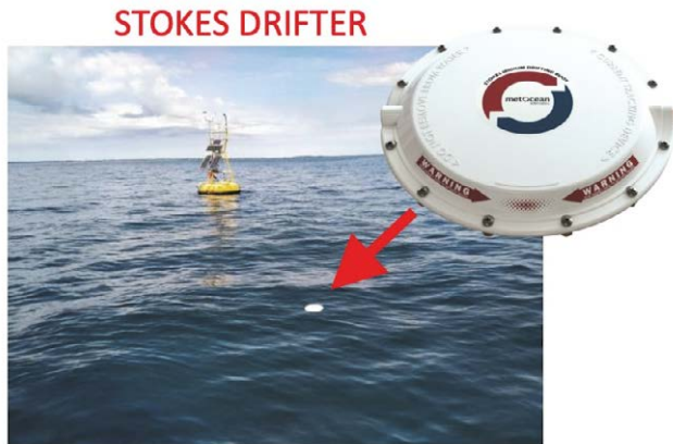
Figure 5 – Picture of a drifter released in the water during a model validation test.
