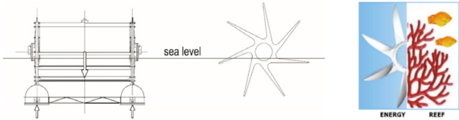
Figure 2 – Impeller close to indifferent equilibrium or in meso-float, similar to jellyfish, so that it can turn even at the slightest sea currents, and the project logo.
