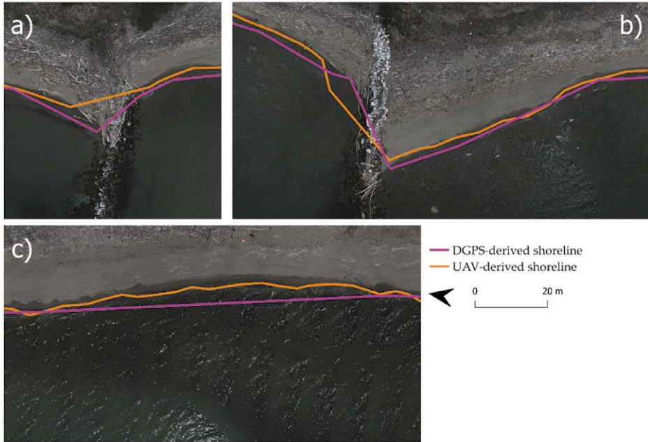
Figure 4 – Shorelines derived from DGPS points (pink line) and from UAV image processing (orange line). a) The DGPS-derived shoreline (pink line) approximates the real shoreline better than the UAV-derived shoreline (orange line); b) the two shorelines approximate the real shoreline better alternating; c) the UAV-derived shoreline (orange line) approximates the real shoreline better than the DGPS-derived shoreline (pink line) (modified by [62]).
