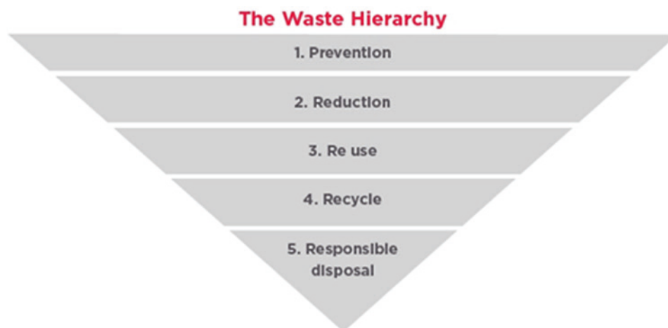
■ Figure 9.10 Hierarchical approaches to waste management guide and rank waste management decisions. The preferred option is the prevention of waste generation, through limiting raw materials or acquiring used/recycled materials or materials that can be recycled. Waste disposal is unsustainable and can have long-term environmental impacts. Disposal is the least preferred option and should be carried out responsibly. Image: Wikibooks: CC-BY-SA-3.0
