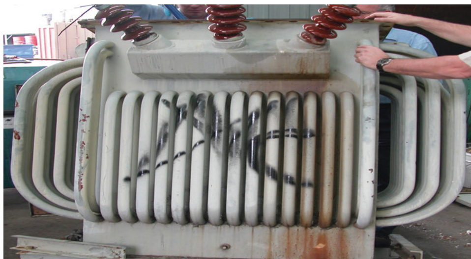
Figure 8.3 Liquid Aroclors (PCB mixtures) had worldwide use as dielectric fluid in transformers common throughout power supply grids. In practice, the dielectric is an oily liquid that surrounds the electricity-conducting copper wire coils inside the transformer. Its roles are cooling and electrical insulation, and both the transformer body and the cooling pipes visible on the outside of the transformer shown here are filled with dielectric fluid. The disposal of these PCB mixtures from obsolete and redundant equipment is an ongoing concern. Poor disposal practices in the past (e.g. to unlined landfill) caused serious widespread contamination of waterways and aquatic ecosystems. Photo: M. Mortimer
