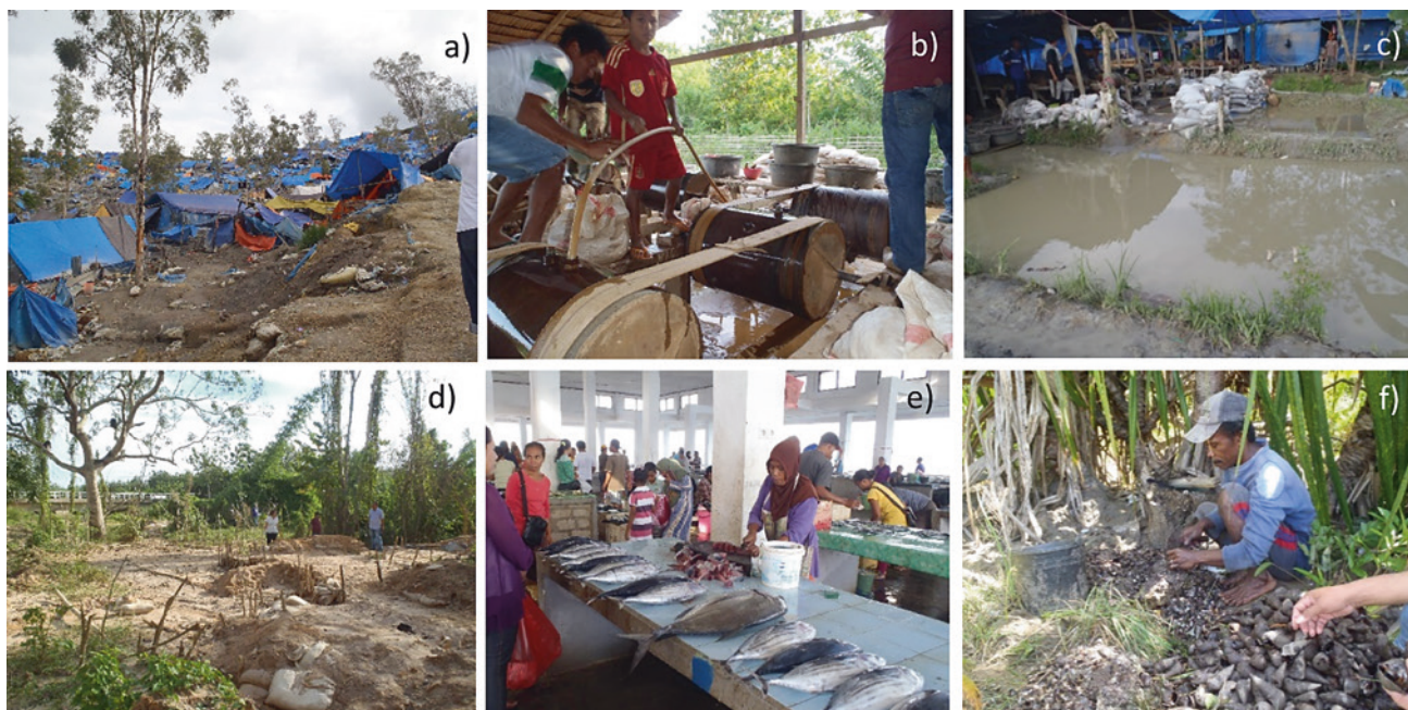
Figure 5.4 Artisanal gold mining and food resources on Buru Island, Eastern Indonesia: a one of the mine sites (Gogrea) in operation; b trommel operations to crush ore and extract the with mercury. Water is used to flush the spent ore to the tailings ponds, c tailings ponds are designed with small trenches to overflow to the river, d abandoned trommel operations on the Wae Apu River bank, e up to 90% of protein comes from the marine environment in many areas of Eastern Indonesia, Buru Island fish markets, f wild harvest of mangrove molluscs. Photos: A. Reichelt-Brushett
