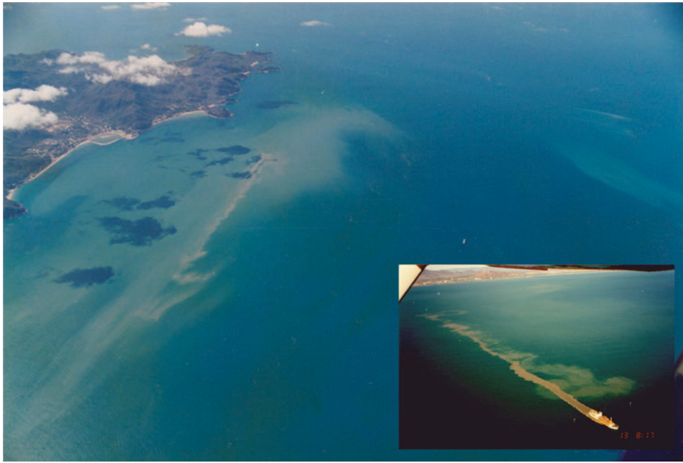
■ Figure 12.5 Capital dredging works in Platypus Channel, Cleveland Bay, Australia in 1991 (insert bottom right). In the main picture suspended sediments can be seen drifting from the dredge site to the shores of Magnetic Island. The trailing suction hopper dredge in action. Photos: Dredging Assessment Project Team, James Cook University, 1991
