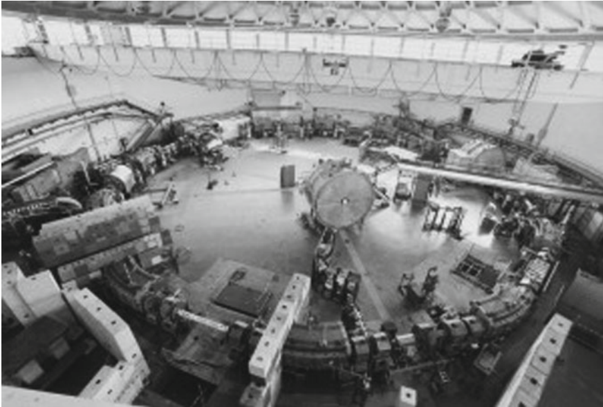
Fig. 16.5 ADONE in its building during assembly. The circumference is 100 m, the magnet bending radius 5 m and the energy 1.5 GeV. The injector is a 300 MeV electron linac built by Varian, with the capability of positron injection rate of 10 mA/minute. The design required 100 mA per beam to reach the design luminosity of about 3 \times 10^{32} \text{ cm}^{-2} \text{ h}^{-1}
