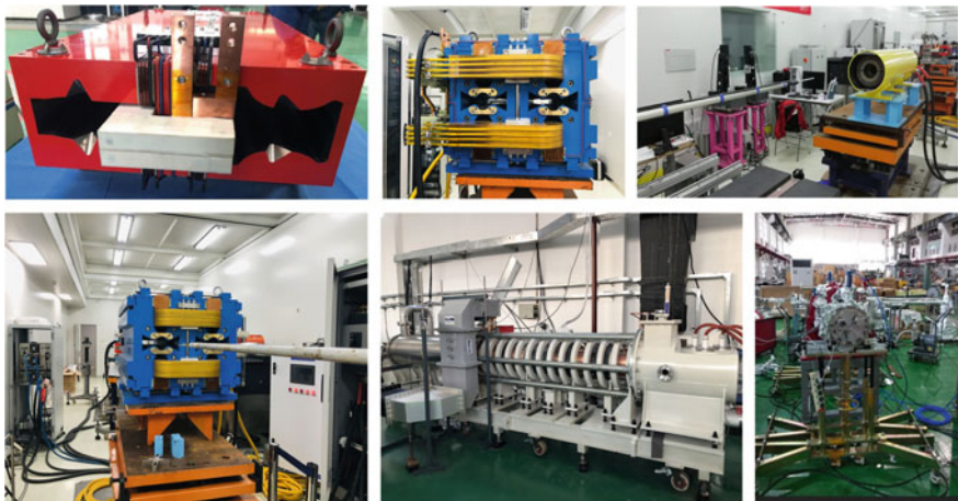
Fig. 21.5 Prototypes of magnets, electro-static separator, Klystrons, vacuum pipes with NEG coating, etc. for CEPC (photos IHEP)
