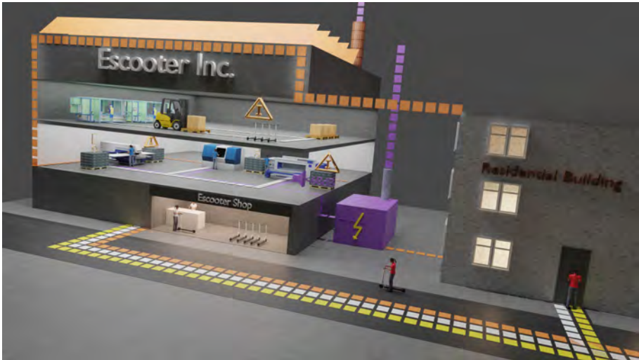
Fig. 1. Mockup of an AR UP scene with production and distribution close to the customers. In the scenario, both interconnection (highlighted purple emissions, orange energy, yellow people, white material) and value stream planning combined with sector coupling (utilisation of process heat and excessive energy for private residences) are based on [16]
