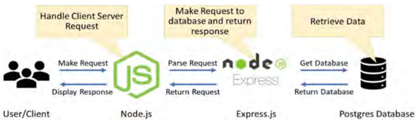
Fig. 4. 'Smart DMIE' dashboard web-based application and language architecture
