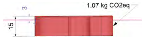
Fig. 2. Suggestion for a 3 mm reduction in height of the original CAD model to reduce CO 2 eq
