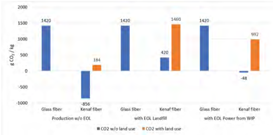
Fig. 3. Comparison of CO 2 emissions of glass fiber and kenaf fiber without and with accounting for land use as a missing CO 2 reservoir for 1 year.
