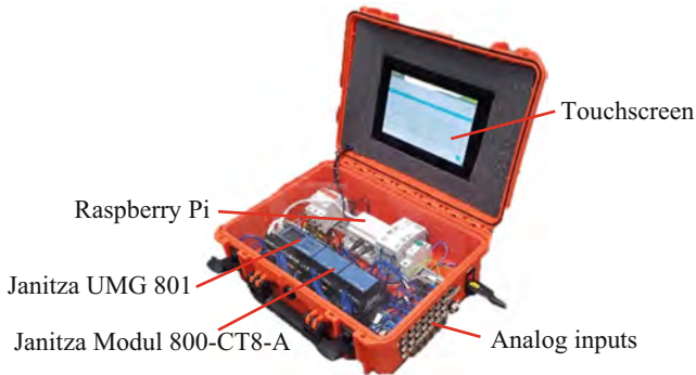
Fig. 2. Energy transparency and analysis system (ETAS).
