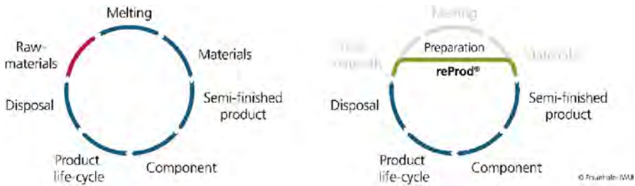
Fig. 3. The standard metal cycle and the smart shortened reProd ® cycle by cutting off the most energy-consuming and CO 2 -emitting process steps, such as melting and hot rolling.
