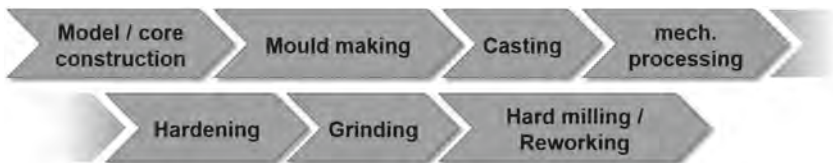
Fig. 3. Process chain for manufacturing the tool with cast cooling channels/sand core casting, based on [4]
