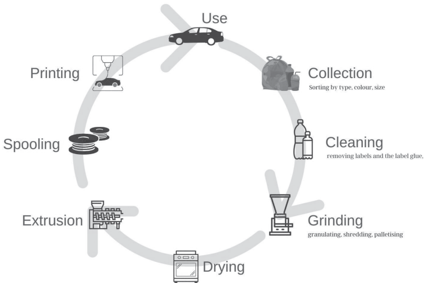
FIGURE 6.1 The basic steps of converting waste to 3D-printed products (Oyinlola et al., 2023)
