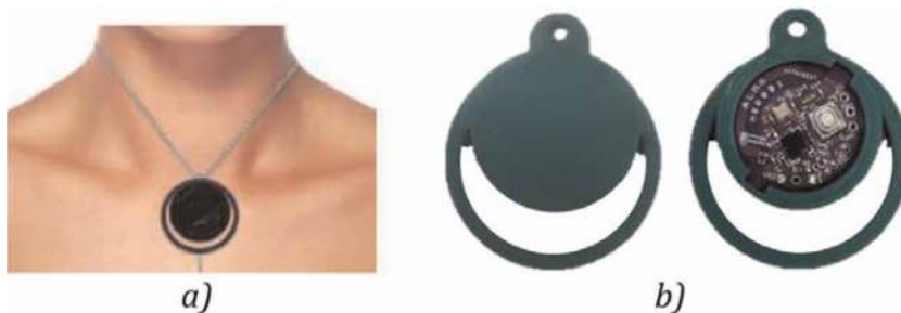
Figure 8. Appearance of the necklace: a) proposed design and b) thermoplastic prototype with the hidden device.
